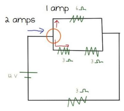
Two amps are flowing into the node I picked, and 1 amp is flowing out of the node into the top branch. So, 1 amp must be flowing into the bottom branch.
