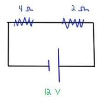
The 12 volts is across the whole circuit, not just one of the resistors. So, before we find the current, we need to add the resistors together to get the total resistance:
