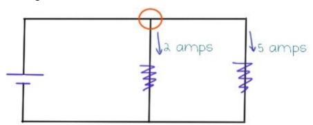
2 amps and 5 amps are flowing out of that node and into the resistors, so 7 amps must be flowing in.
