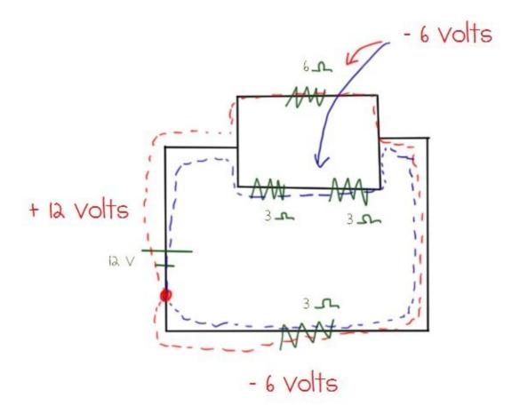
Let's start with the top resistor. There is a voltage drop of 6 volts across it, and it has a resistance of 6 ohms. We can use ohm's law to find the current:
