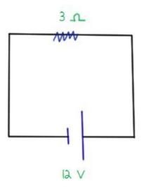
The voltage across the resistor is 12 volts, the resistance is 3 ohms. We plug that into our equation:
