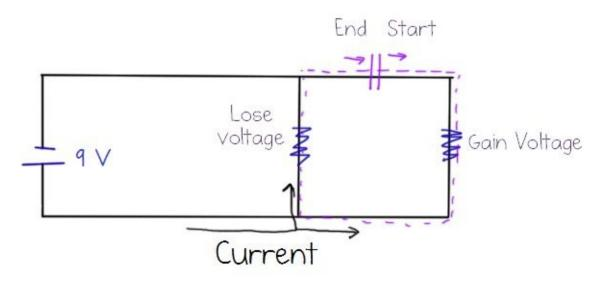
If you go through a resistor in the same direction as the current, you lose voltage. If you go through the resistor against the current, you gain voltage.
