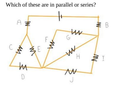
Check your Answer: E is parallel to CD, H is parallel to FG and IJ. A and B are in series with CDE and FGHIJ.
