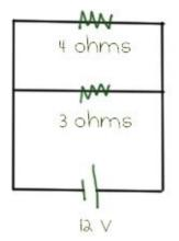
First, we need to know the voltage across each of the resistors. Taking two loops, we can see that the voltage must be 12 volts across each.
