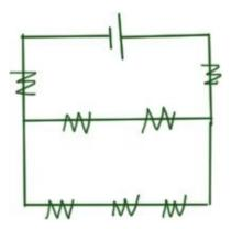
Keep in mind that sometimes if you redraw a circuit diagram, it will make the problem easier to solve. A good way to do this is to aim for putting all resistors on horizontal lines.
