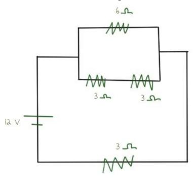
The first thing we need to do is figure out the total resistance. First we'll add the two in series:
