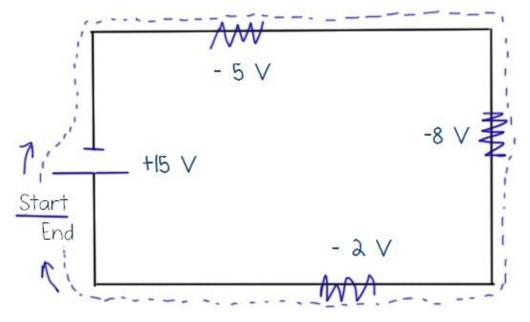
Notice that we gain voltage across the battery, and lose voltage going across the resistors. Here's the equation we would write for this:
