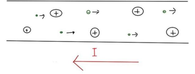
The symbol for current is I, and it is measured in Amps, which are Coulombs per Second. (Because current is flowing charge, it is measured in the amount of charge (coulombs) that flow through the wire per second.
