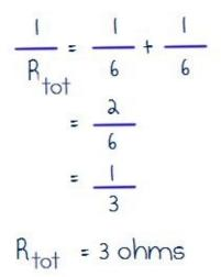
Now the circuit looks like this (because we replace the two 6 ohm resistors with 1 3 ohm resistor):
