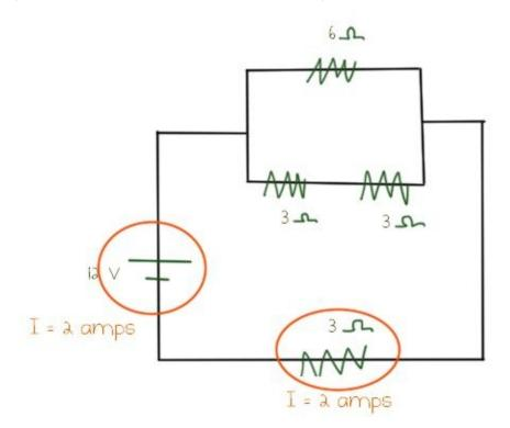
Now we need to find the current through the other three resistors. To do this, we need to know the voltage drop across that piece of the circuit. Since we know the current and resistance of the lower resistor, we can figure out the voltage drop using ohm's law:
