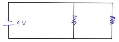
The voltage drop must be 9 volts across each of the resistors. Here are the two loops we could draw:
