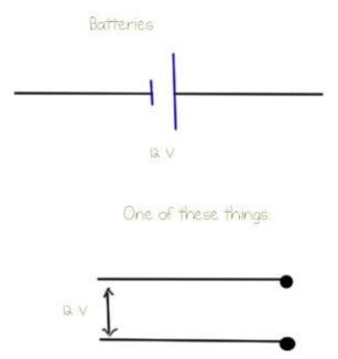
The second one just means that the difference in potential energy per unit charge between the top ball and the bottom ball is 12 volts. It's exactly the same as if there were a battery there, we just don't know where the voltage difference is coming from. (Like, is there a generator there? A battery? Little fairies carrying charges around?)
