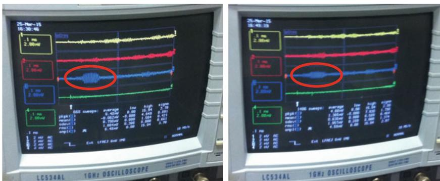
**Fig. 3** Results of the signal acquisition phase: the FSAT was excited with a 10 cycles sinusoidal burst around 78 kHz. The presence of the mass is evident on the right hand side image where a noticeable decrease in signal amplitude is present
