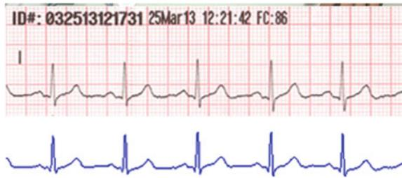
keep. The signals are clean and free of artifact due to muscular activity. Furthermore, a comparison of the first lead of the ECG signal recorded using simultaneously the prototype (i.e. by placing the hands on its electrodes) and a professional ECG monitor (i.e. by attaching wet electrodes on the chest) confirms that the signals are very similar and can be overlapped almost perfectly, as shown in Fig. 5.
