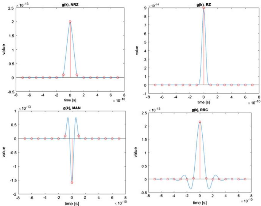
Fig. 3 Plots of  $g(t)$  and  $g(k)$  for the four pulse shapes taken into account in the paper
