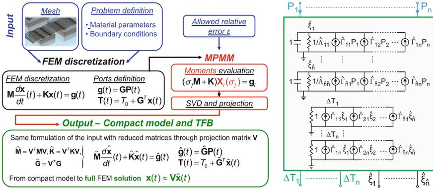
Fig. 1 Proposed TFB extraction procedure (left) and topology (right)
