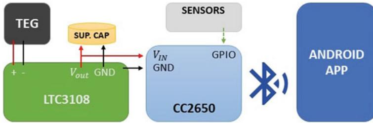
**Fig. 2** Block scheme of the proposed solution
