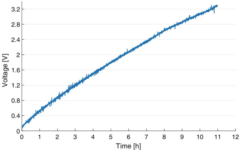
**Fig. 9** Super-capacitor charge with the TEG
