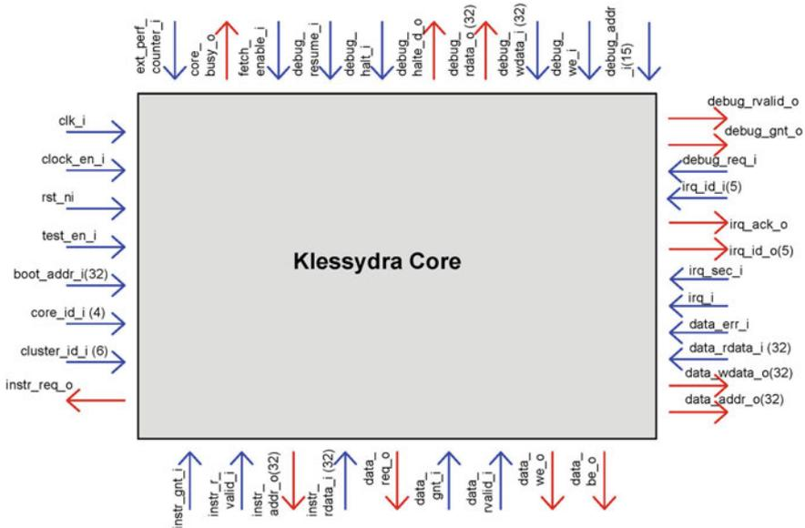
**Fig. 2** Klessydra processing core pinout
