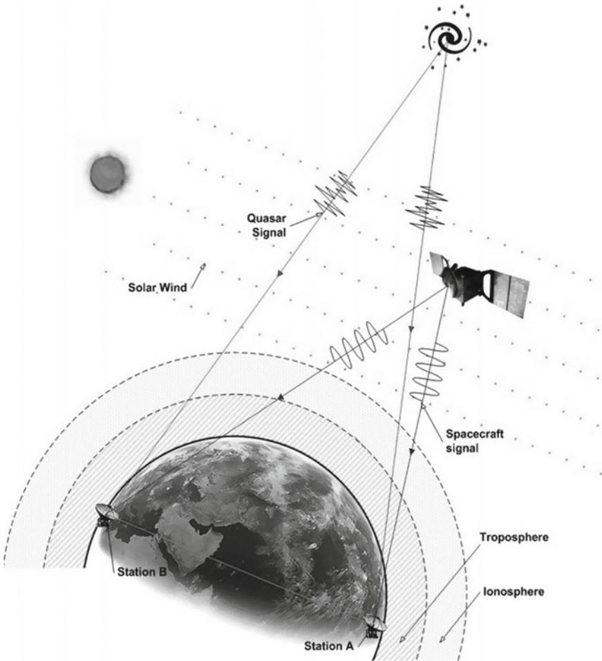
**Fig. 1**  $\Delta$ DOR geometry
