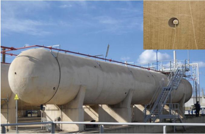
**Fig. 3** AE method on a tank
