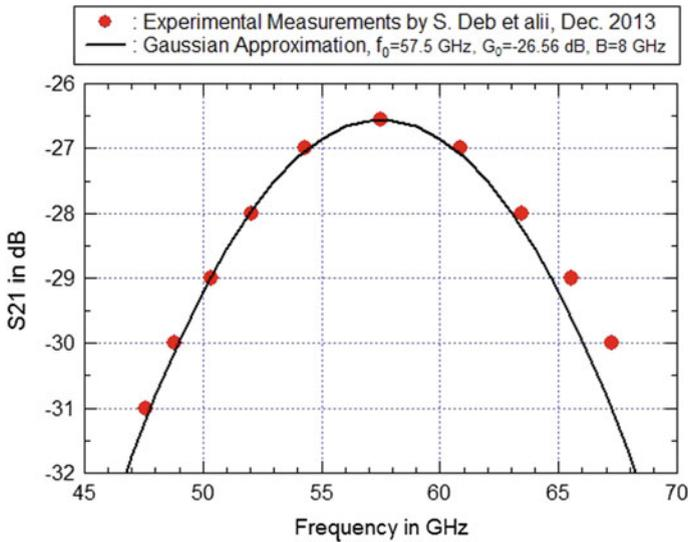
Fig. 2 Approximation of the antenna gain with a Gaussian gain shape
