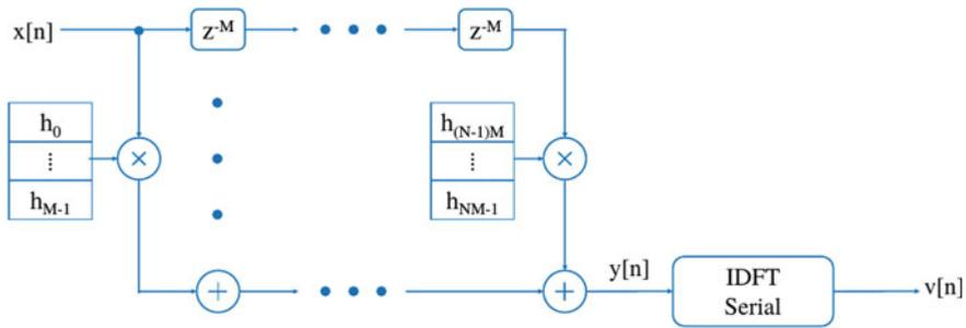
**Fig. 2** Serial implementation of digital filter bank
