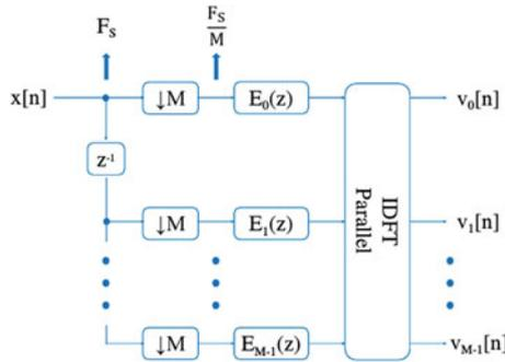
Fig. 1 Multistage implementation of digital filter bank
