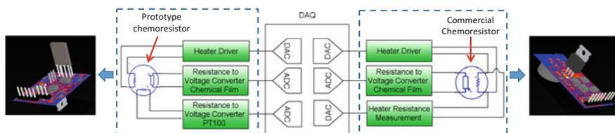
**Fig. 3** Front end block diagrams for prototype (left) and commercial (right) chemoresistive sensors
