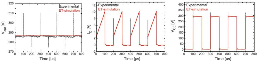
**Fig. 4** ET (solid) versus measurement data (dots) for the boost steady-state behavior
