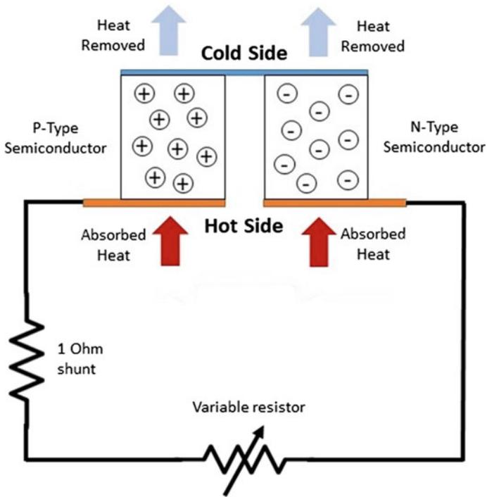
**Fig. 3** Working principle of a thermoelectric generator and load setup
