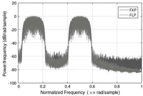
**Fig. 6** Wideband and narrowband DOR signals
