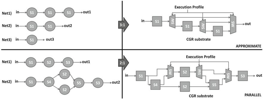
Fig. 1 Dataflow to hardware: Trade-off friendly CGR platforms
