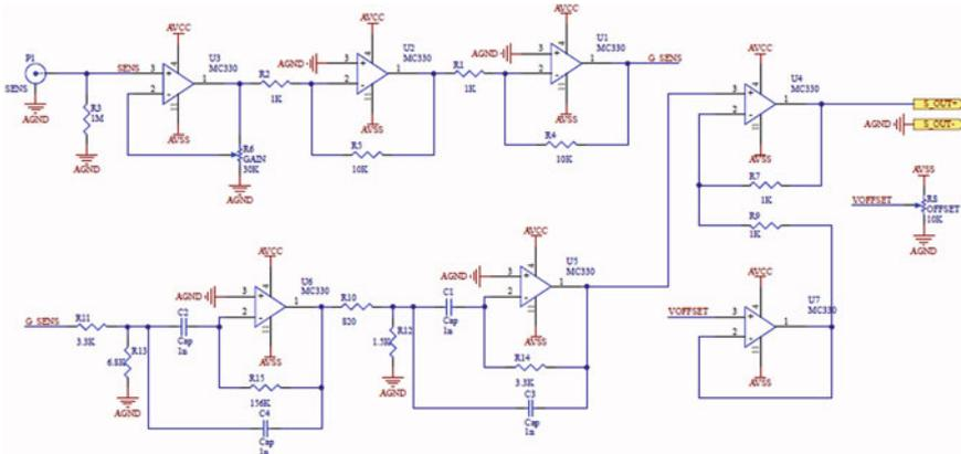
Fig. 4 Analog conditioning circuit
