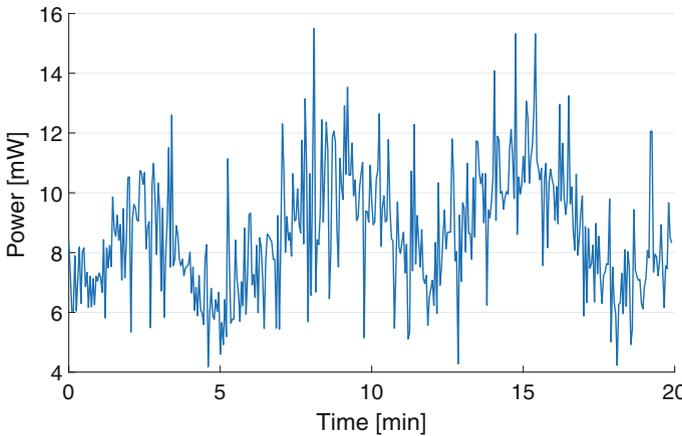
Fig. 6 Output power with 10°C temperature gradient
