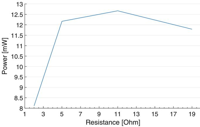
Fig. 5 Power characterization at different load conditions
