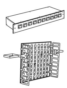
Figure 18.4 Data network patch-panel hardware.
