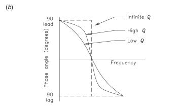
**Figure 6.10** Characteristics of a series resonant circuit as a function of frequency for a constant applied voltage and different circuit Qs: (a) magnitude, (b) phase angle.
