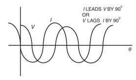
**Figure 6.8** Waveforms representing leading and lagging phasors. (*From* [2]. *Used with permission*.)
