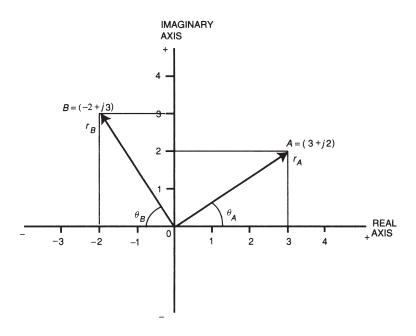
**Figure 6.6** The *s* plane representing two complex numbers. (*From* [2]. *Used with permission*.)
