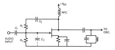
Figure 16.6 Simplified reactance modulator. (From [1]. Used with permission.)
