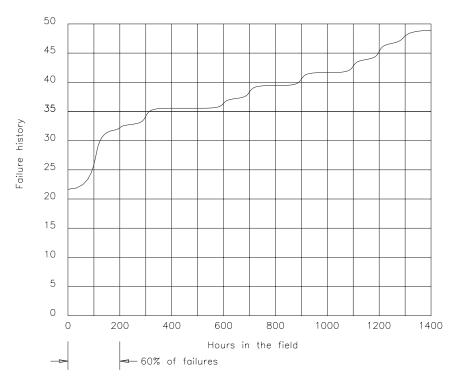
**Figure 20.4** The failure history of a piece of avionics equipment vs. time. Note that 60 percent of the failures occurred within the first 200 hours of service. (*After* [1].)
