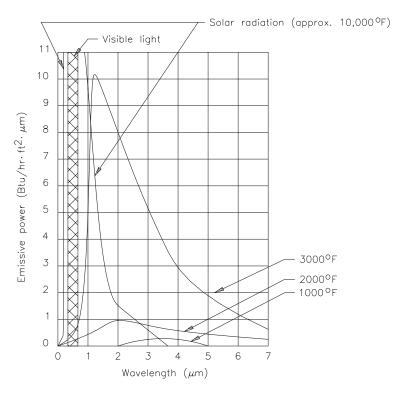
Figure 11.1 Blackbody energy distribution characteristics.
