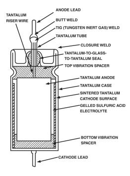
Figure 8.3 Basic construction of a tantalum capacitor.
