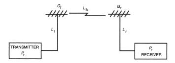
Figure 3.1 Path loss variables. (From [2]. Used with permission.)
