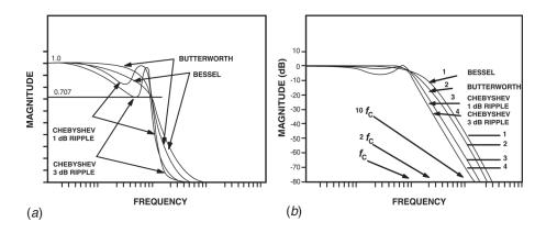
**Figure 10.2** Filter characteristics by alignment, third-order, all-pole filters: (a) magnitude, (b) magnitude in decibels. (*From* [1]. *Used with permission*.)
