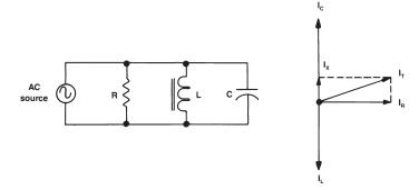
Figure 6.5 Current vectors in a parallel RLC circuit.
