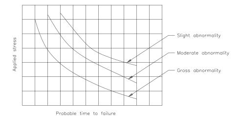
**Figure 20.9** Estimation of the probable time to failure from an abnormal solder joint. (*After* [5].)
