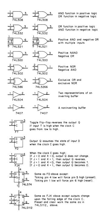
Figure 14.6 Symbols used in digital system block diagrams.
