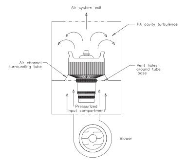
$\textbf{Figure 11.5} \ \ \textbf{A poorly designed cooling system in which circulating air in the output compartment reduces the effectiveness of the heat-removal system.}$
