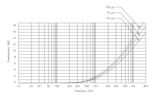
Figure 16.4 Preemphasis curves for time constants of 50, 75, and 100  $\mu$ s.
