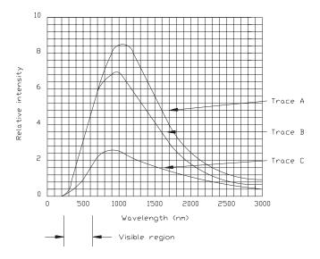
**Figure 5.2** The typical radiating characteristics of tungsten: (trace A) the radiant flux from 1 cm<sup>2</sup> of a blackbody at 3000 K, (trace B) radiant flux from 1 cm<sup>2</sup> of tungsten at 3000 K, (trace C) radiant flux from 2.27 cm<sup>2</sup> of tungsten at 3000 K (equal to curve A in the visible region). (*After* [1].)
