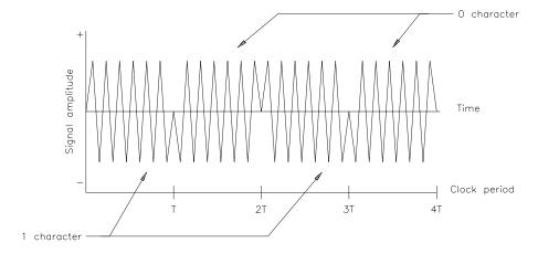
Figure 17.7 Binary PSK waveform.
