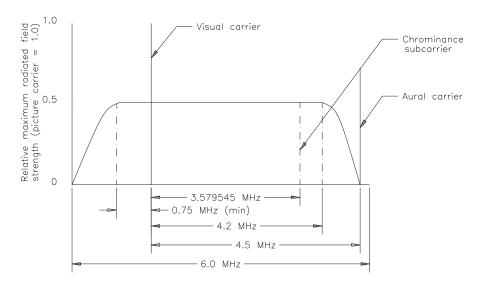
**Figure 15.4** Idealized amplitude characteristics of the FCC standard waveform for monochrome and color TV transmission. (*Adapted from*: FCC Rules, Sec. 73.699.)
