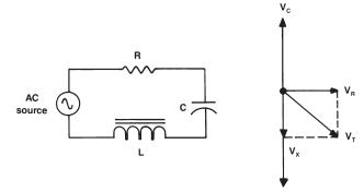
Figure 6.4 Voltage vectors in a series RLC circuit.
