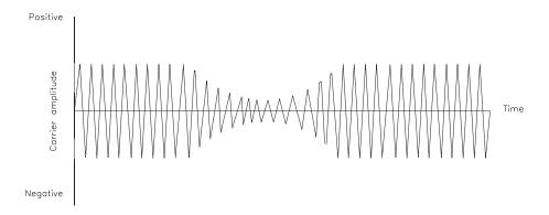
**Figure 15.2** Time-domain representation of an amplitude-modulated signal. Modulation at 100 percent is defined as the point at which the peak of the waveform reaches twice the carrier level, and the minimum point of the waveform is zero.
