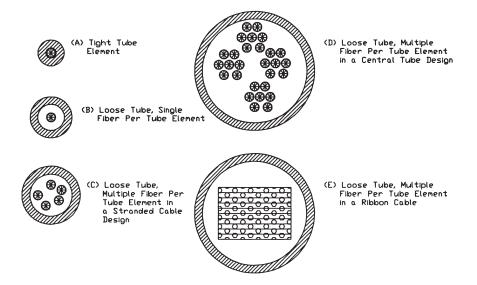
**Figure 19.3** Loose-tube cables are available in either single-fiber-per-tube (SFPT) or multiple-fibers-per-tube (MFPT) designs. In both cases, the diameter of the plastic tube surrounding the core is larger than the outside diameter of the core. In a tight tube cable; the inner diameter tube is the same as the outer diameter of the fiber.
