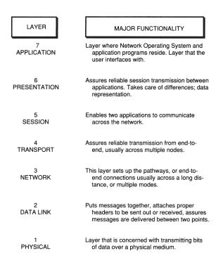
Figure 18.1 The OSI reference model.
