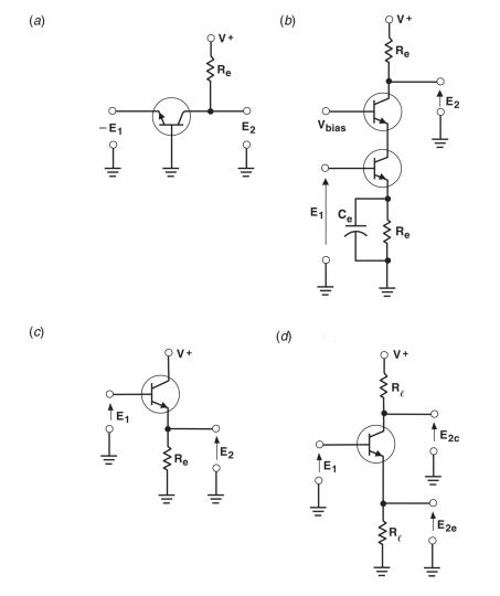
**Figure 13.3** Transistor amplifier circuits: (*a*) common-base NPN, (*b*) cascode NPN, (*c*) common-collector NPN emitter follower, (*d*) split-load phase inverter.
