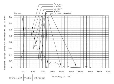
**Figure 5.3** Spectral distribution of solar radiant power density at sea level, showing the ozone, oxygen, and carbon dioxide absorption bands. (*After* [1].)
