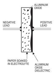
**Figure 8.5** Failure mechanism of a leaky aluminum electrolytic capacitor. As the device ages, the aluminum oxide dissolves into the electrolyte, causing the capacitor to become leaky at high voltages.
