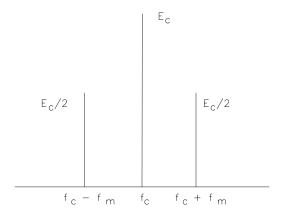
**Figure 15.1** Frequency-domain representation of an amplitude-modulated signal at 100 percent modulation.  $E_c$  = carrier power,  $F_c$  = frequency of the carrier, and  $F_m$  = frequency of the modulating signal.
