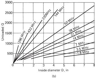
**Figure 10.4** Helical resonators: (a) round and square shielded types, showing principal dimensions (diameter D or side S is determined by the desired unloaded Q), (b) unloaded Q versus shield diameter D for bands from 1.8 MHz to 1.3 GHz. (From [3]. Used with permission.)
