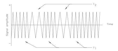
Figure 17.6 Binary FSK waveform.
