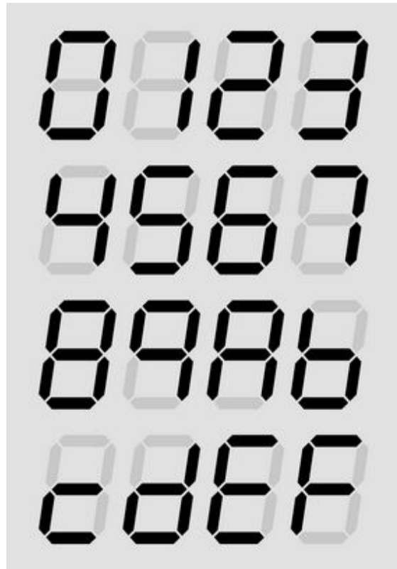
Figure 17-5. Numerals and the first six letters of the alphabet created with a 7-segment display.
