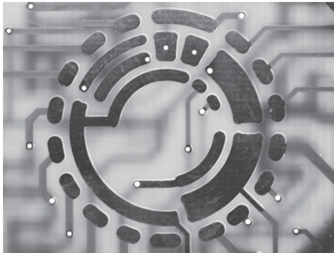
FIGURE 10-11 Rotary switch contacts, back illuminated
