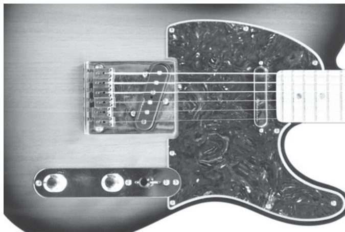
FIGURE 12-2 Electronic elements of the Telecaster
