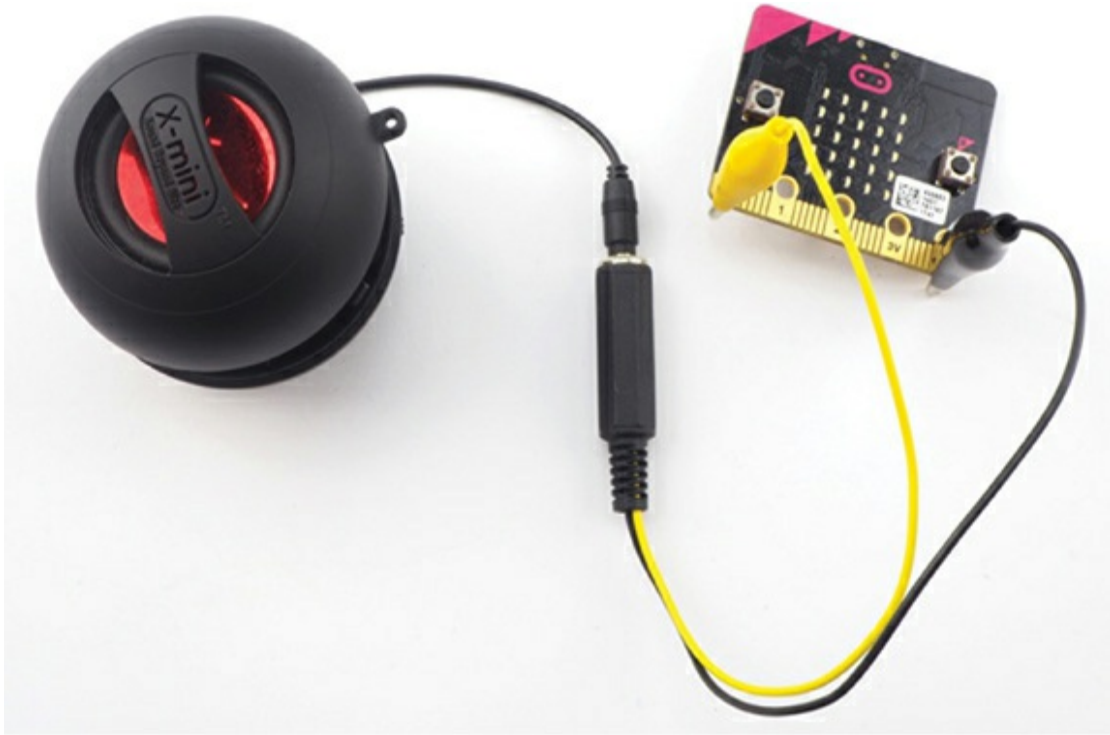
Figure 2-3: Connecting a micro:bit to an amplified speaker
