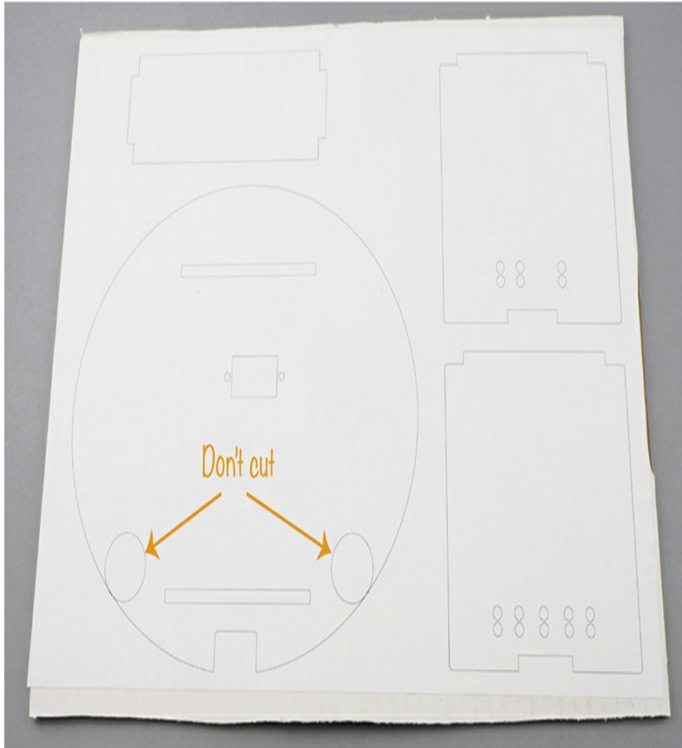
Figure 6-10: The paper template glued to a piece of cardboard
