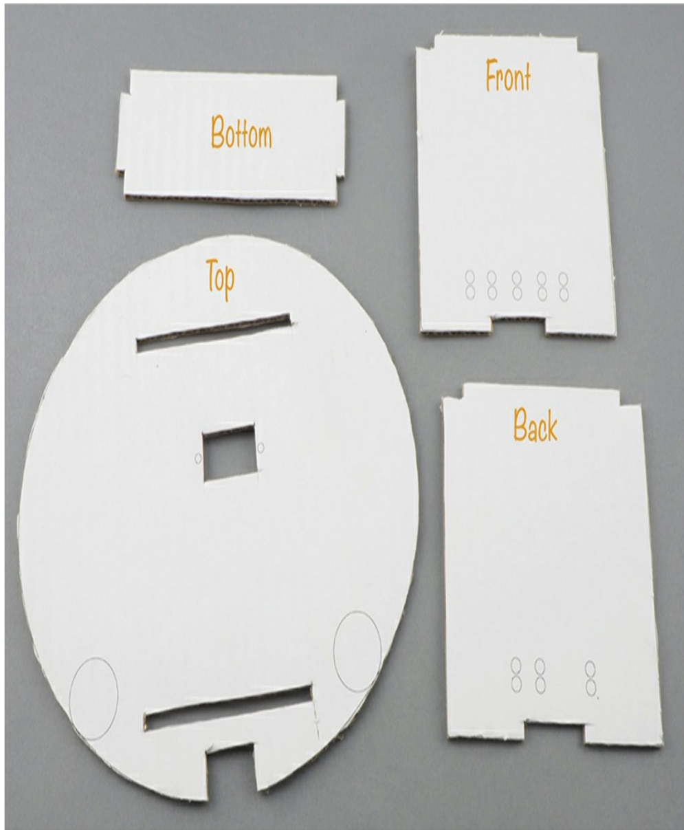
Figure 6-11: The cardboard pieces for the chassis
