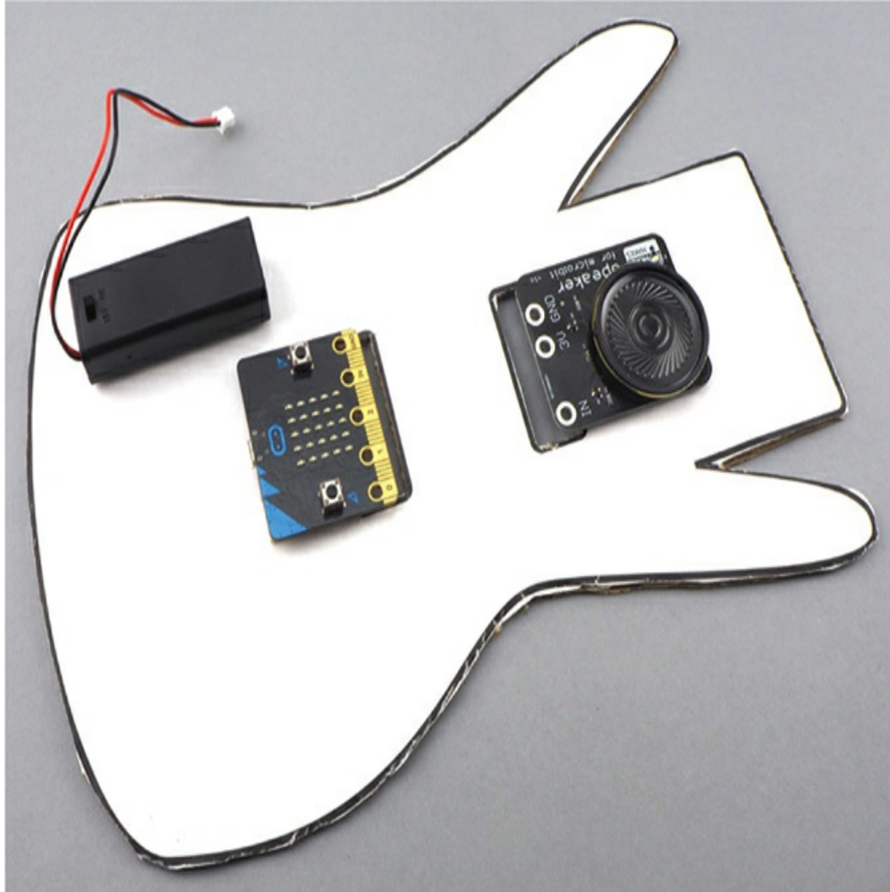
Figure 3-6: The micro:bit, speaker, and battery box have been attached to the guitar.
