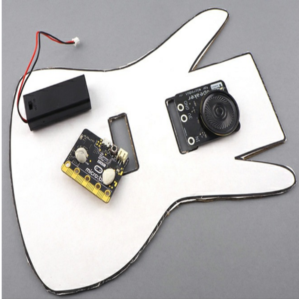
Figure 3-5: Attaching the micro:bit, the speaker, and the battery box
