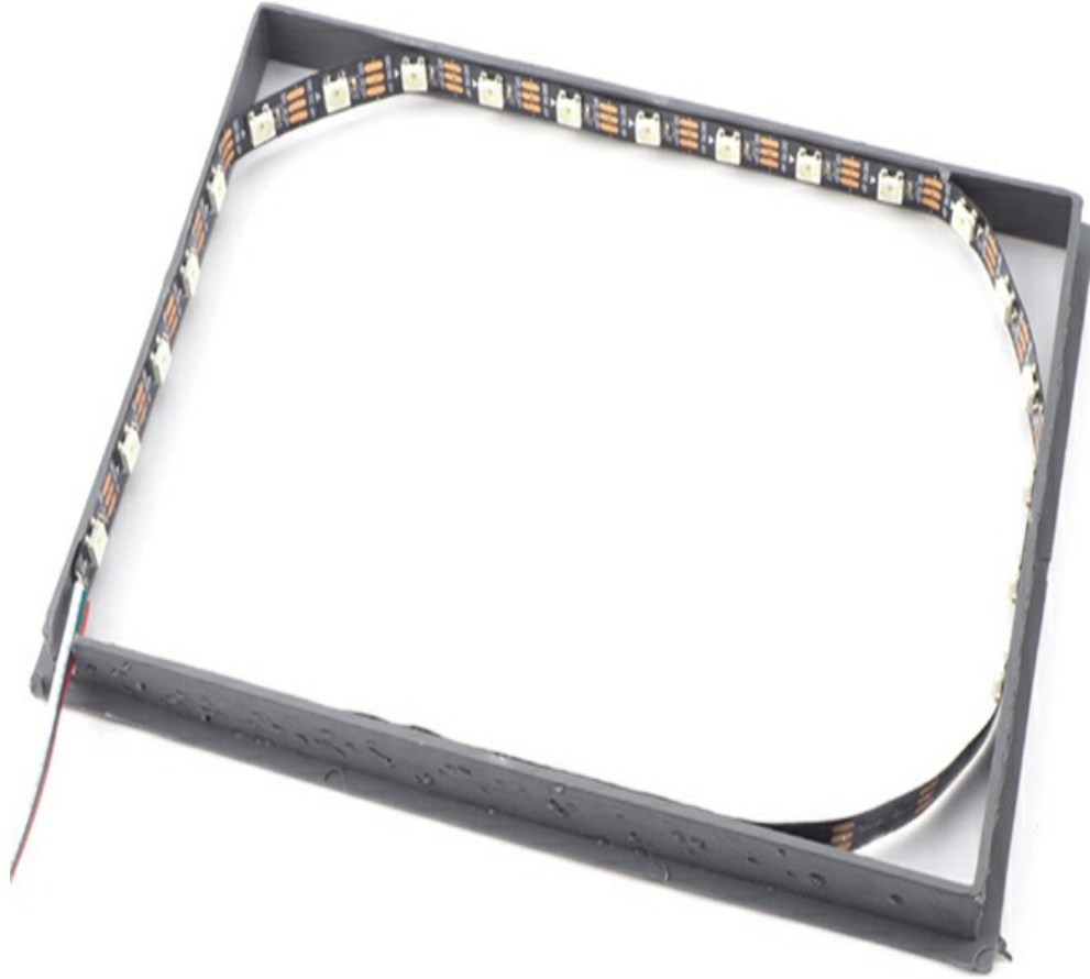
Figure 3-13: Attaching the LED strip to the plastic insert
