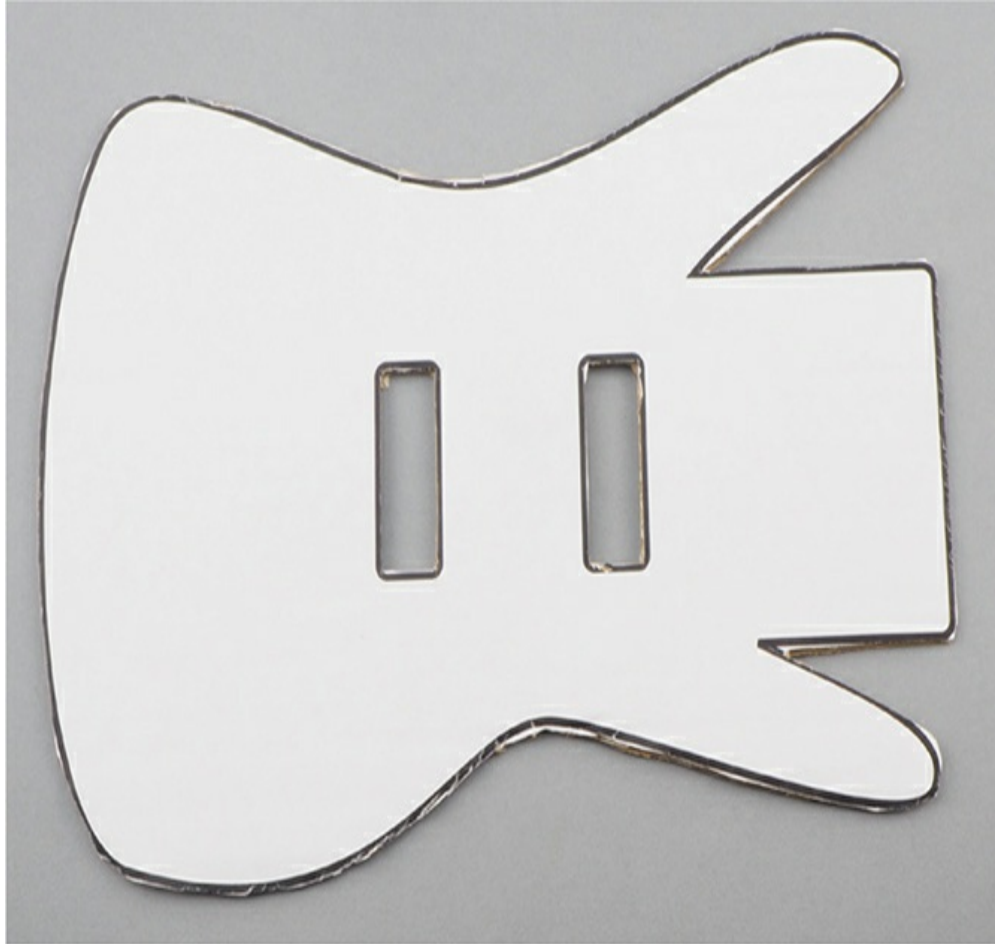
Figure 3-4: Cutting around the template
