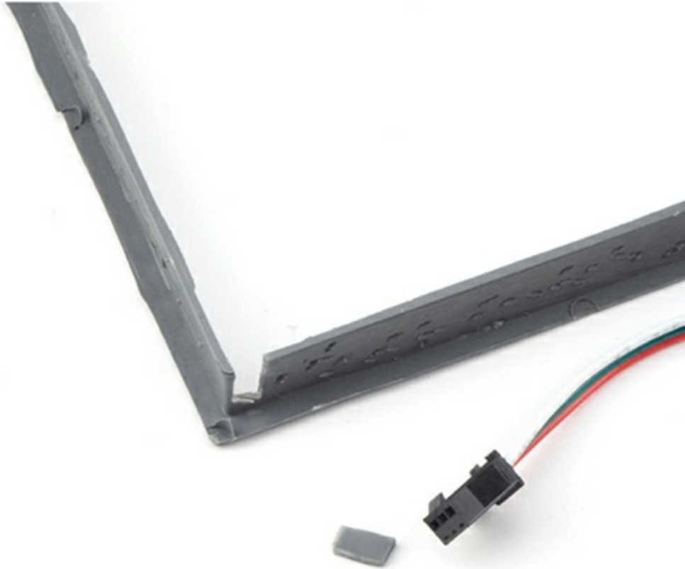
Figure 3-12: Cutting a groove for the wires in the plastic insert
