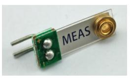
FIGURE 8-10 A piezo vibration sensor
