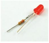
FIGURE 6-20 Making an LED resistor combo
