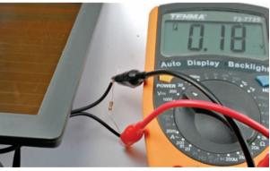
FIGURE 5-14 Testing a solar panel
