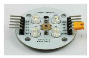
FIGURE 8-7 A light-sensing module
