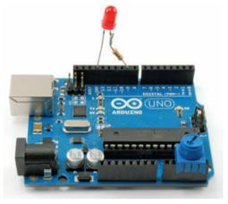
FIGURE 6-19 An Arduino, variable resistor, and LED
