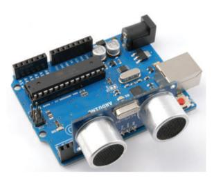
FIGURE 7-9 An HC-SR04 rangefinder on an Arduino
