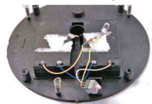
FIGURE 3-20 Replacing the bulb with an LED and a resistor
