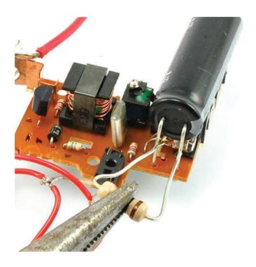
FIGURE 10-1 Safely discharging a capacitor
