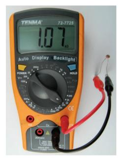
FIGURE 3-8 Measuring the LDR resistance
