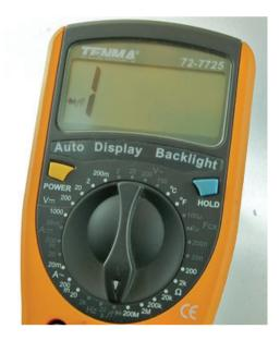
FIGURE 1-8 A multimeter in Continuity mode
