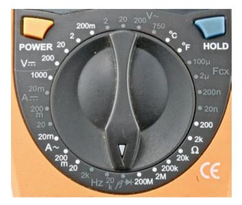
FIGURE 11-1 Multimeter range selection
