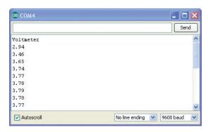
**FIGURE 6-18** The Serial Monitor showing voltage at A3
