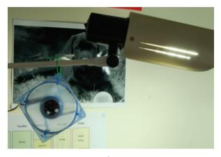
Figure 1-10 A homemade fume extractor
