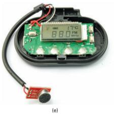
FIGURE 9-11 Modding the FM transmitter
