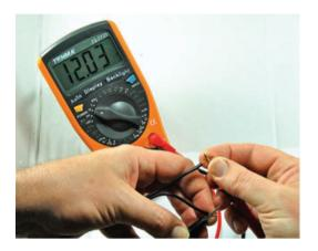
FIGURE 1-13 Using a multimeter to find the power supply polarity
