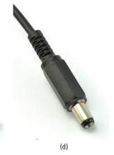
FIGURE 10-7 Attaching a barrel jack to a cell phone charger
