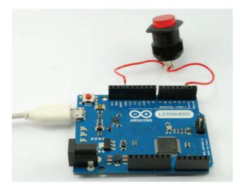
FIGURE 6-35 Entering passwords automatically with Arduino Leonardo
