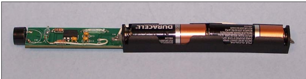
PCB and battery assembly
