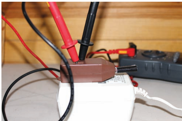
FIGURE 5-10 A severed block tap keeps high voltage from exposed prongs. You can insert the meter probe tips into the outlet slots.
