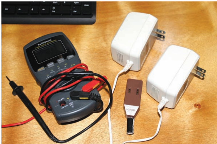
FIGURE 5-7 Devices for transformer experiments: Multimeter, hacked extension cord outlet, and two adapters that convert 120-V AC utility electricity to either 18 V AC or 24 V AC (Radio Shack part number 273-0331 or equivalent).
