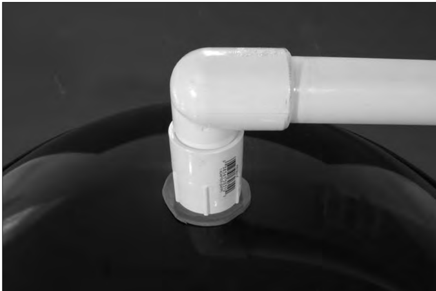
Figure 6-11: Fittings assembled on the parabolic dish.
