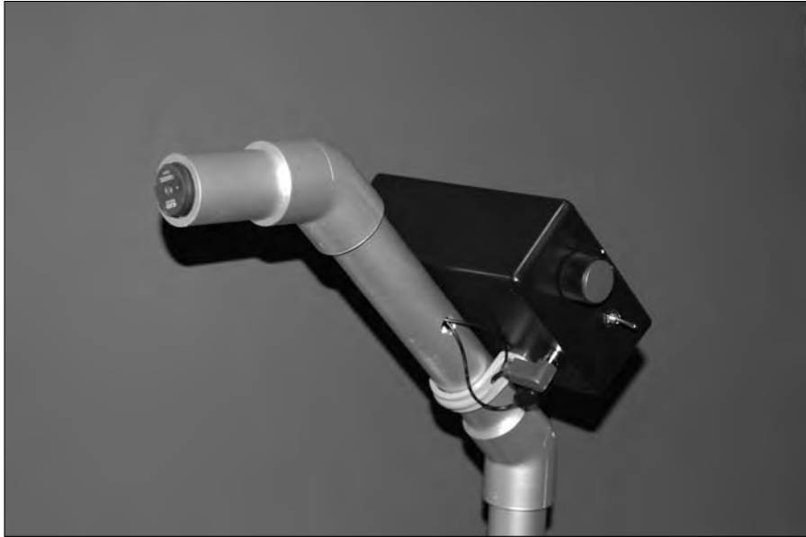
Figure 12-18: The finished metal detector.
