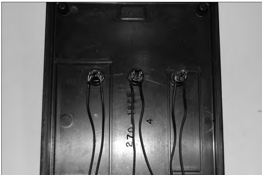
Figure 11-18: Attach wires to the switches.
