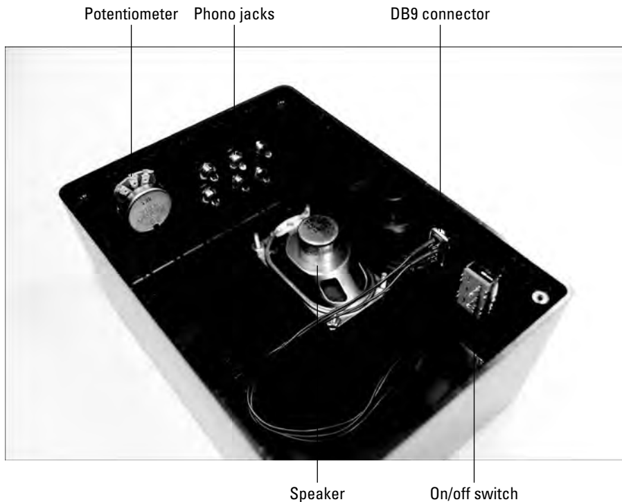
Figure 7-11: Mount components on the box.
