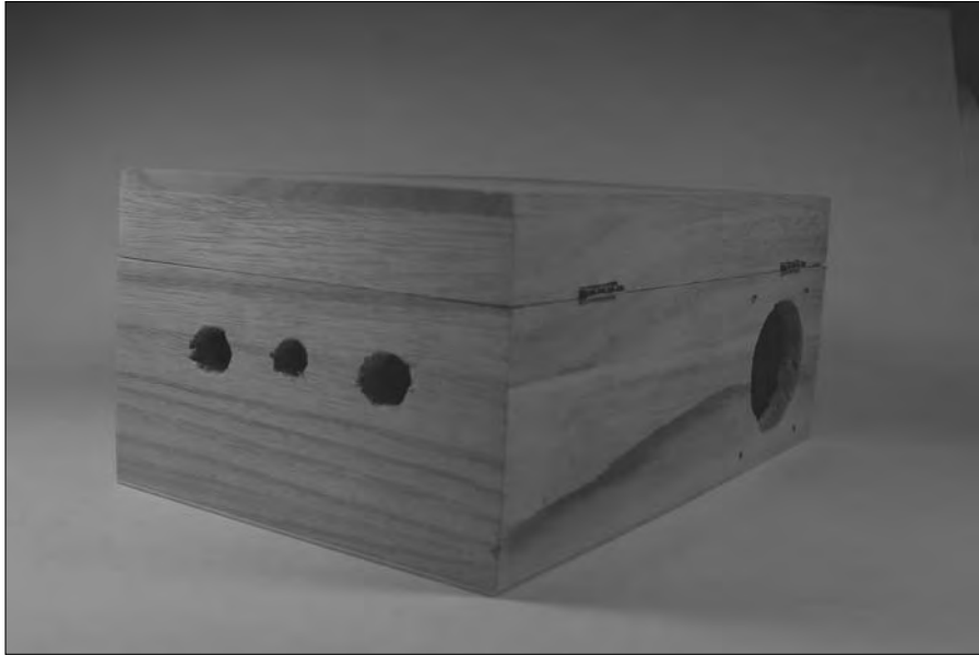
Figure 14-9: Drill holes for the switches, microphone, and speaker.
