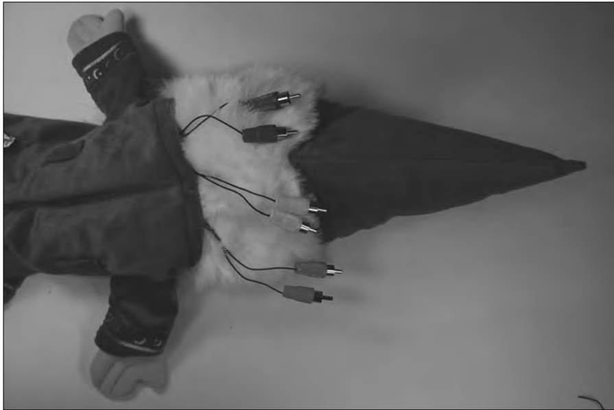
Figure 7-18: Place tactile switches in the puppet.
