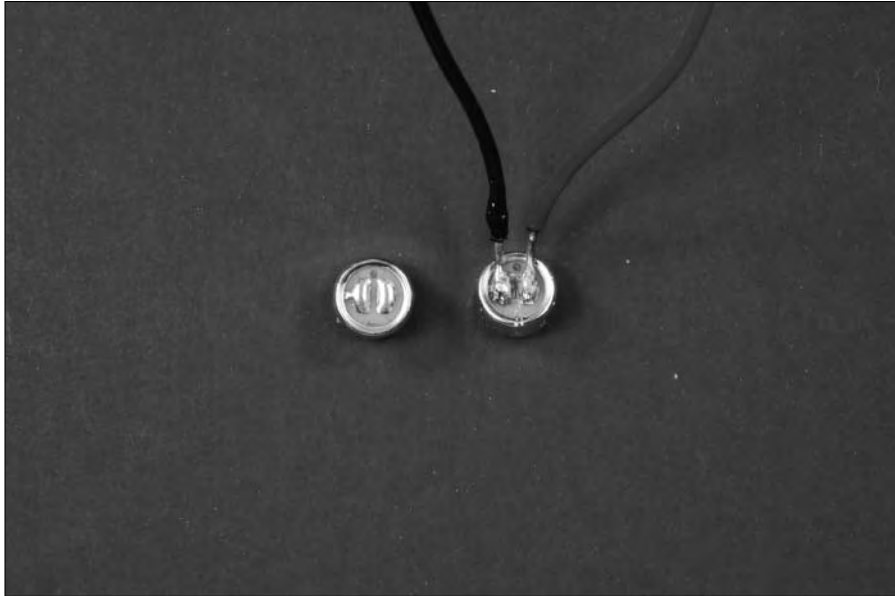
Figure 4-14: Soldering to flat contact pads.
