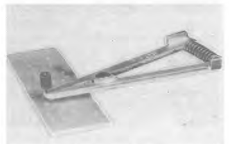
Figure 7 Some sensitive components may need a heatsink
