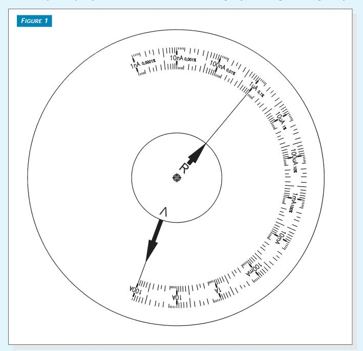
This wheel, using transparent material, gives current values of 1 nA to 100A.
