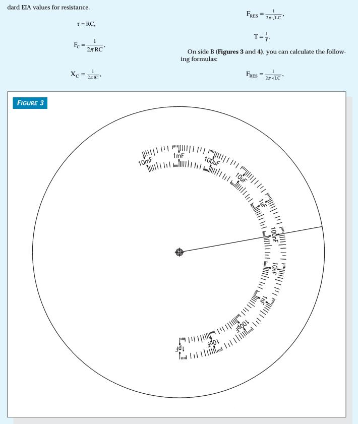
This wheel, copied onto transparency material, gives capacitance values from 1 pF to 10 mF (10,000 µF).
