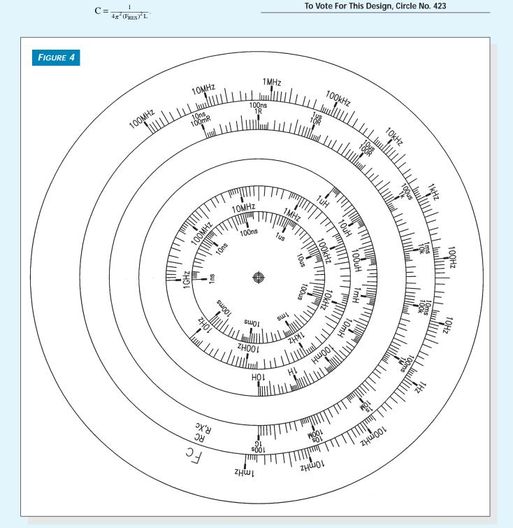
This wheel, the opaque backing for the wheel in Figure 2, relates resistance, frequencies, and time constants to the capacitance values on the wheel in Figure 3.
