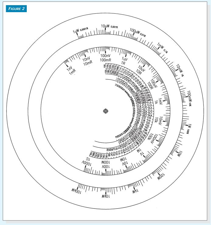
This wheel, an opaque background, gives voltage, current, power, and dissipation-factor percentages. The inner rows give standard EIA resistance values.
