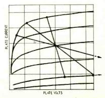
Fig. 11-Pentode characteristic curves.
