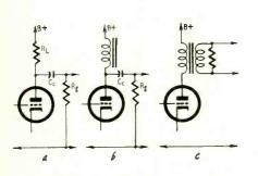
Fig. 9—Typical coupling circuits.
