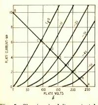
Fig. 5-Showing load line principle.
