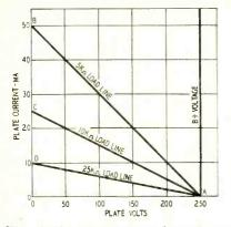
Fig. 7-Comparing load line slopes.
