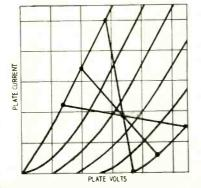
Fig. 10-Typical triode characteristics,
