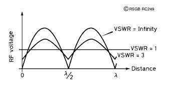
Figure 3 Standing waves on a transmission line
