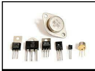
Fig. 2.—Family of bipolar transistors. Some common types that exist in the market can be observed.
