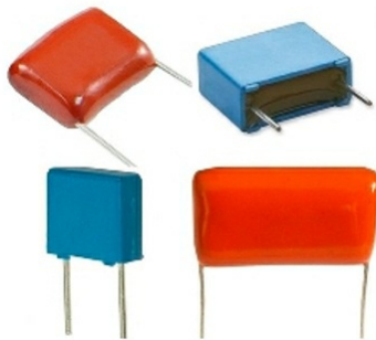
Fig. 3-Plastic or polyester capacitors. The size depends on the capacity and the applied voltage.
