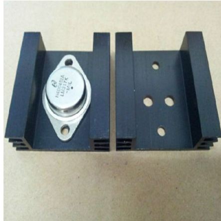
Fig. 2.—Sometimes it is necessary to use large radiators, in this case they dissipate the heat generated by power transistors with TO-3 capsule.
