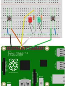
Figure 4-16. Circuit diagram for the robot soccer game
