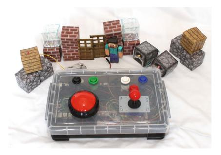
Figure 9-5. Minecraft blocks with tri-color status LEDs
