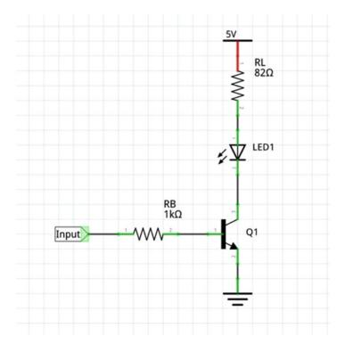
Figure 11-7. Transistor LED circuit schematic view
