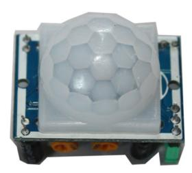
Figure 5-3. PIR motion sensor
