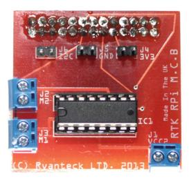
Figure 8-14. Ryanteck Motor Control Board
