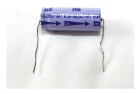
Figure C-2. Electrolytic capacitor
