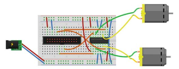
Figure 8-13. Robot motor control circuit on a breadboard
