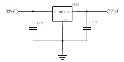
Figure 11-14. 7805 voltage regulator circuit
