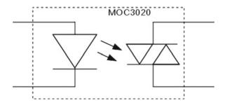
Figure 4-29. Circuit symbol for a TRIAC opto-isolator
