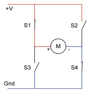
Figure 8-7. H-bridge motor controller in one direction
