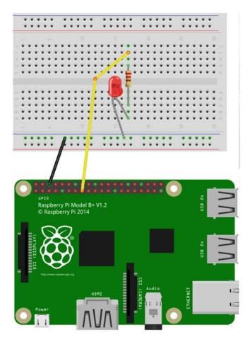
Figure 3-6. LED circuit for Scratch GPIO
