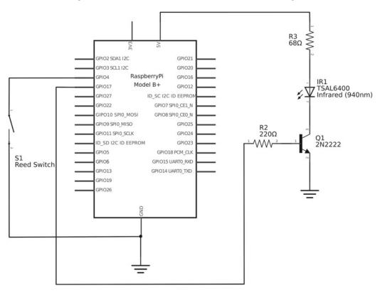
Figure 6-4. Circuit diagram of infrared transmitter with reed switch
