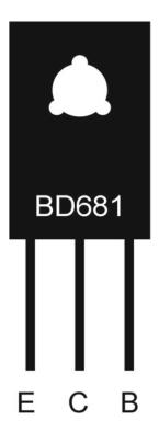
Figure 4-20. BD681 Darlington Transistor pinout
