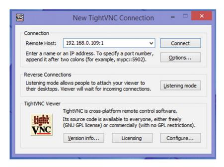
Figure 2-6. Connect remotely using TightVNC
