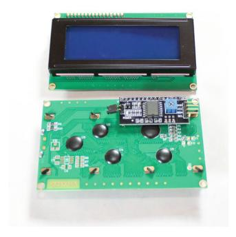
Figure 5-13. Photo of the LCD character display and backpack mounted on the rear
