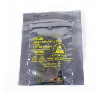
Figure 1-10. Warning symbol for a static-sensitive component
