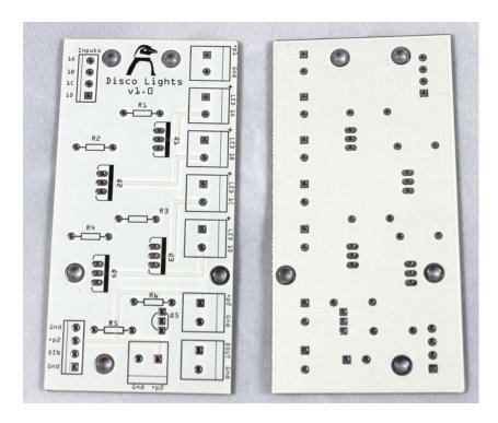
Figure 11-13. Manufactured PCB for disco lights and NeoPixels
