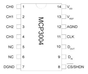
Figure 11-1. Pin layout for the MCP3004
