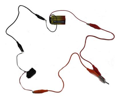
Figure 1-1. Switch and buzzer circuit
