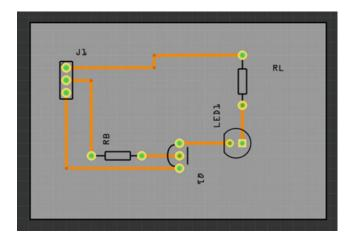
Figure 11-11. PCB layout with copper tracks between the components
