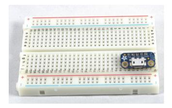
Figure 4-1. A USB power breakout connector
