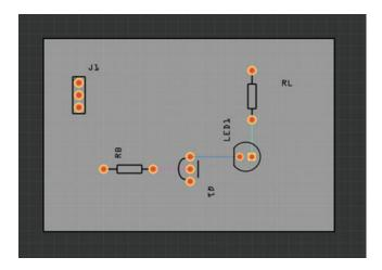
Figure 11-10. Initial PCB layout without routing
