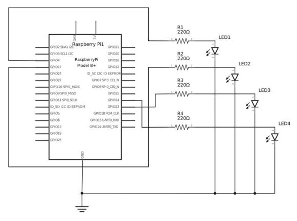
Figure 6-1. Simplified LED disco light circuit
