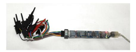
Figure 10-11. BitScope Micro with test leads
