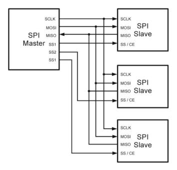
Figure 5-19. SPI bus connections
