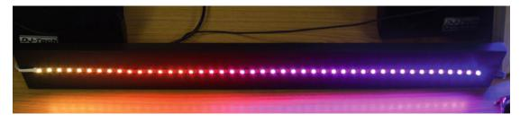
Figure 6-7. Color light strip using RGB LEDs
