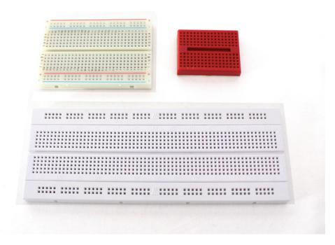
Figure 1-3. A selection of different breadboards
