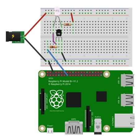
Figure 4-7. Breadboard layout for the bright LED circuit
