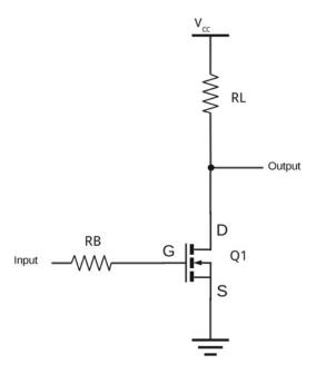
Figure 5-9. MOSFET-based voltage shift buffer
