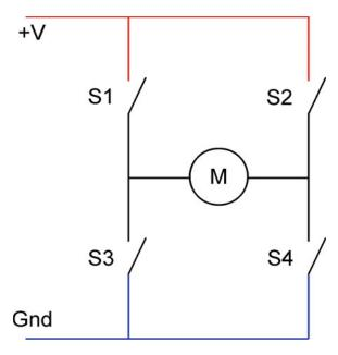
Figure 8-6. H-bridge motor controller in the off position
