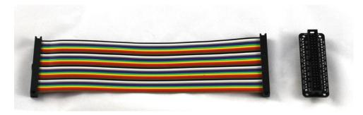
Figure 1-7. Raspberry Pi cobbler (40pin)
