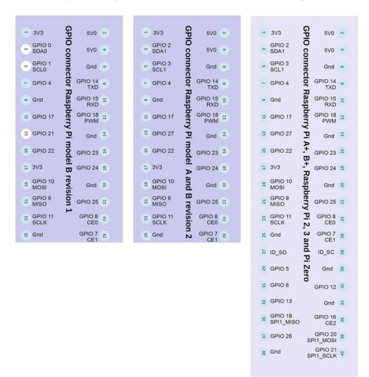
Figure 2-2. Pin layouts for the GPIO for various models of the Raspberry Pi
