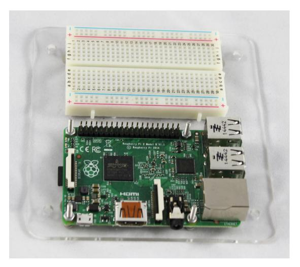
Figure 1-5. Raspberry Pi and a breadboard mounted together
