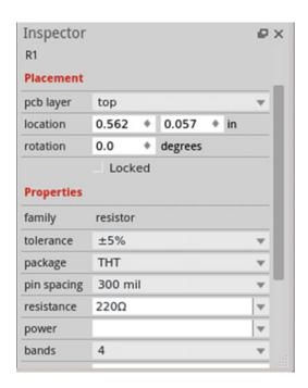
Figure 11-6. Fritzing inspector panel for a resistor
