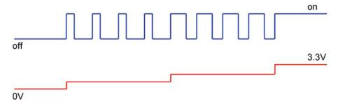
Figure 8-11. Analog output voltage using PWM
