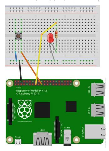
Figure 3-9. Switch and LED circuit
