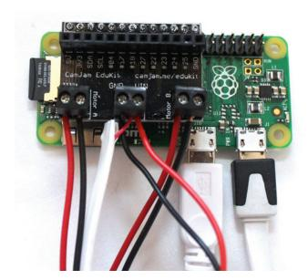
Figure 8-15. CamJam Robotics motor control board
