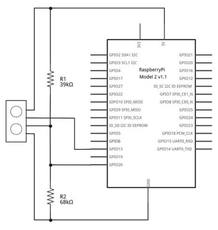
Figure 8-18. Circuit diagram for ultrasonic range sensor
