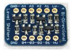
Figure 5-10. Adafruit bidirectional level-shifter
