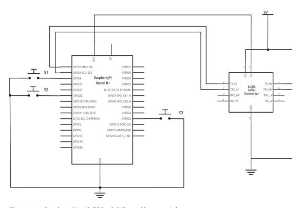
Figure 5-16. Raspberry Pi with I<sup>2</sup>C level-shifter and button switches
