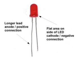
Figure 3-4. A typical LED
