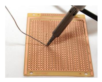
Figure 10-4. Soldering iron just before making a solder joint
