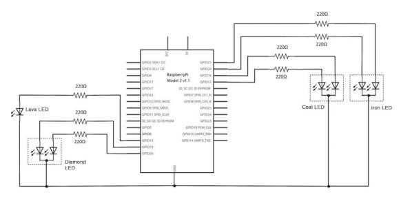
Figure 9-6. Circuit diagram showing tri-color status LEDs
