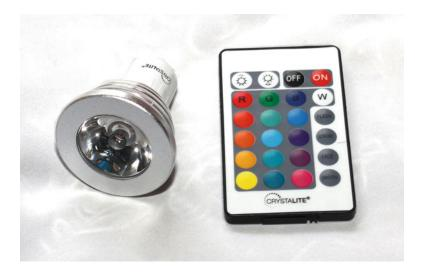
Figure 5-7. Infrared color-changing LED bulb and remote control
