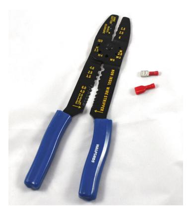
Figure 3-23. Crimp tool with female blade connectors
