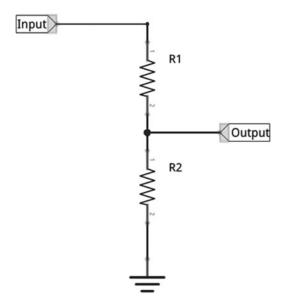
Figure 5-8. Voltage divider circuit
