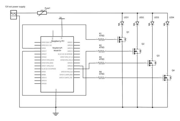
Figure 4-26. Disco light circuit
