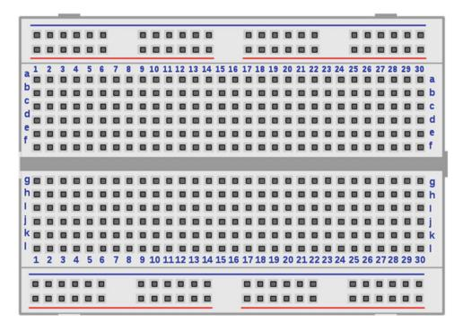
Figure 1-4. A half-size breadboard
