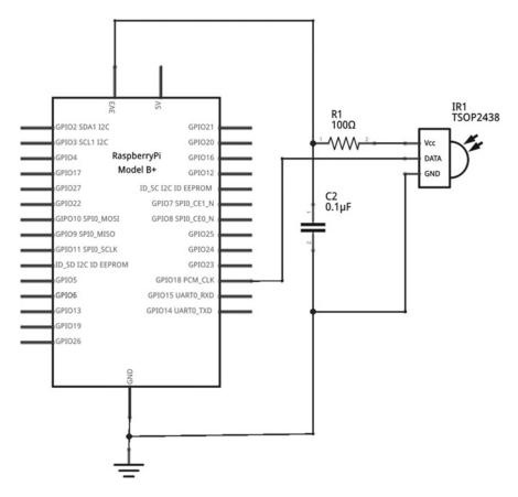
Figure 7-1. Circuit diagram for the infrared receiver circuit
