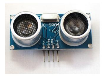
Figure 8-17. Ultrasonic range sensor
