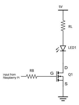
Figure 4-25. MOSFET switch circuit
