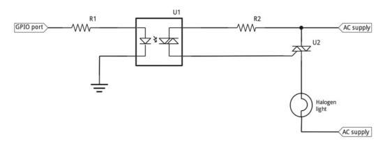
Figure 4-30. Circuit diagram of an AC TRIAC circuit
