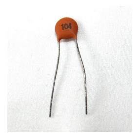
Figure C-4. Ceramic capacitor
