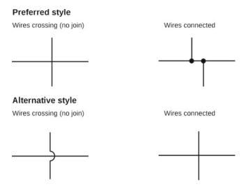
Figure 4-15. Circuit diagram representation of crossing and connecting wires
