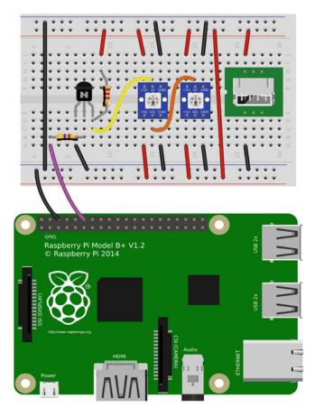
Figure 6-9. Breadboard version of the NeoPixel circuit
