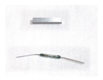
Figure 6-3. A reed switch with magnet
