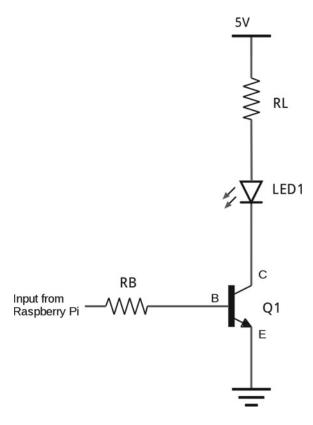
Figure 4-6. Circuit diagram for a transistor switch
