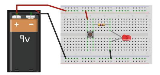
Figure 1-8. Simple LED circuit
