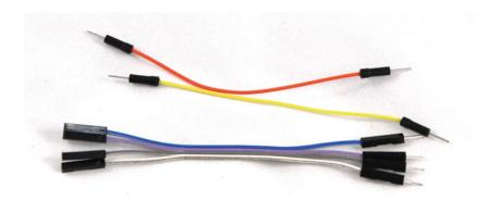
Figure 1-6. Jumper wires—male-to-male and male-to-female
