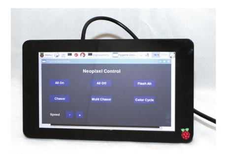
Figure 6-12. Raspberry Pi touch screen running neopixel-gui application
