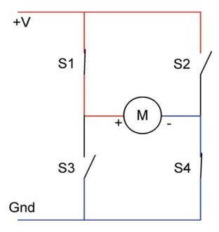
Figure 8-8. H-bridge motor controller in the opposite direction
