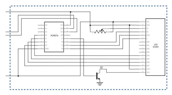
Figure 5-15. LCD display with I<sup>2</sup>C backpack
