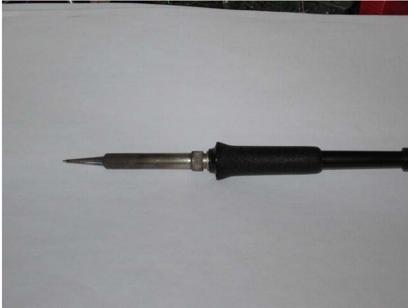
Figure 2-12. The pencil-grip style of soldering irons is better suited for working on small electronics projects.
