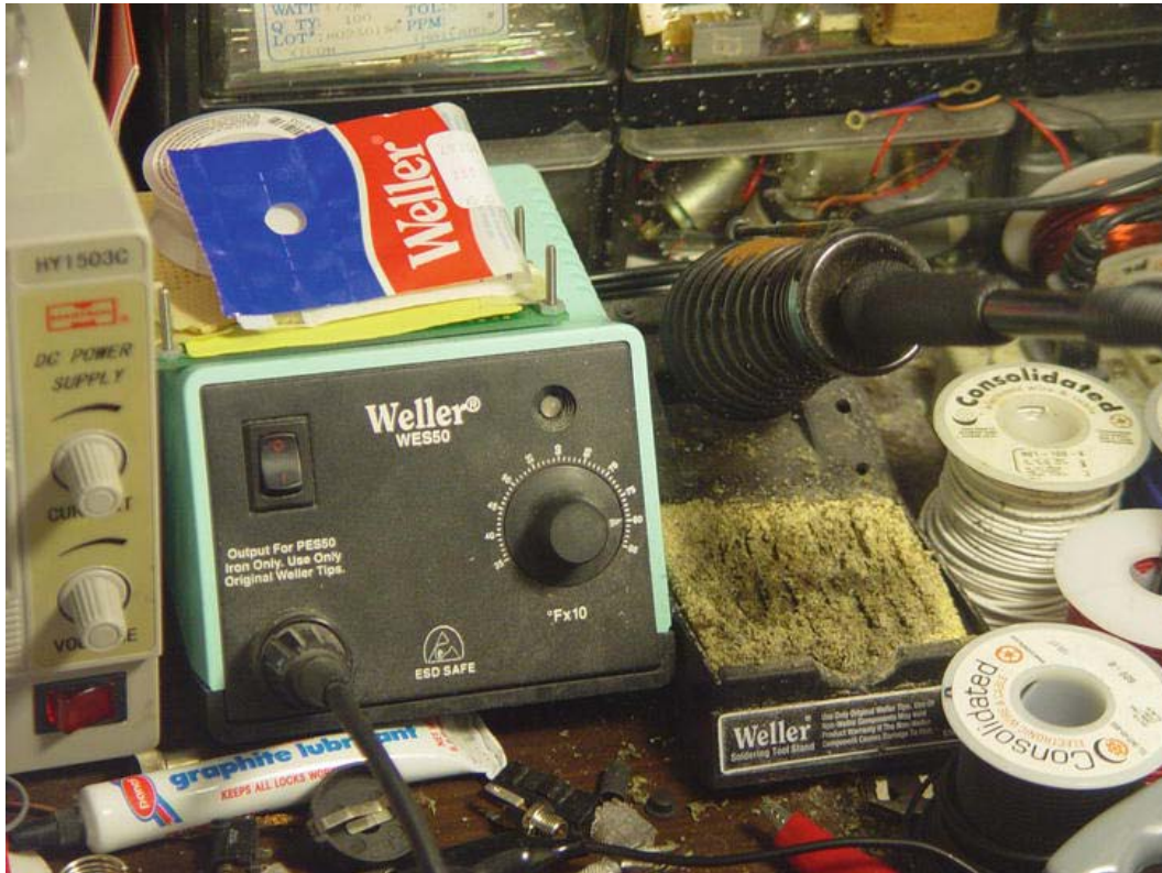
Figure 2-10. A Weller controlled-temperature soldering station. What a mess!
