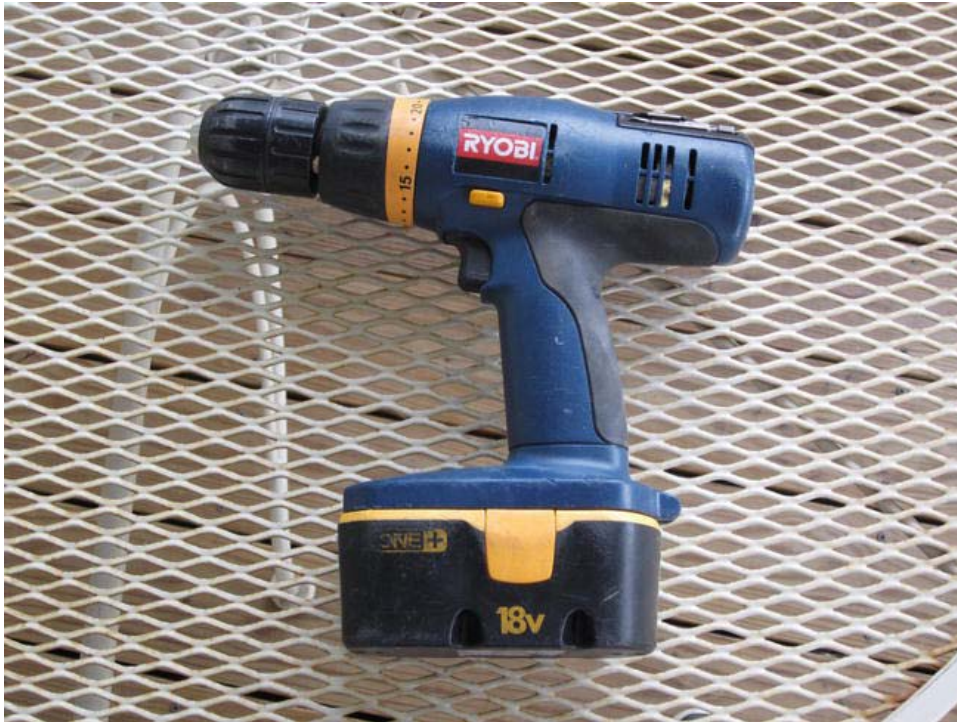
Figure 2-13. A rechargeable hand drill. This model is both variable speed and reversible, which are two very desirable features in a hand drill.
