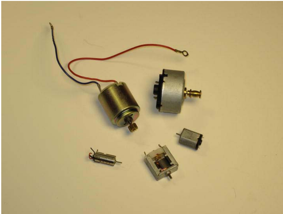
Figure 3-17. Some simple DC motors. When direct current is applied to their terminals, they spin. The magic happens with an electrical and mechanical arrangement inside that performs the necessary commutation of the magnetic fields.
