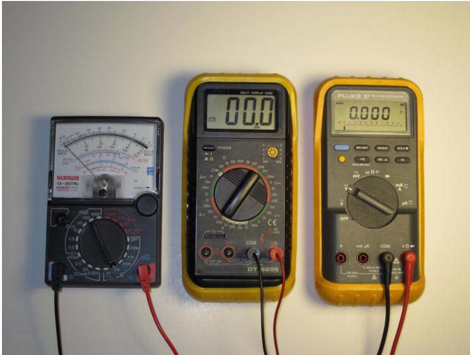
Figure 2-21. Examples of some multimeters. The meter on the left features an analog display that is easy to read and accommodates several readout scales simultaneously. The remaining two meters have digital readouts and offer more accuracy. All the meters use a large rotary knob for selecting the proper function. The higher-cost unit on the right features auto-ranging, intelligently deciding what range to use. The right two units also have high-impact boots to help protect them in the event of a fall.
