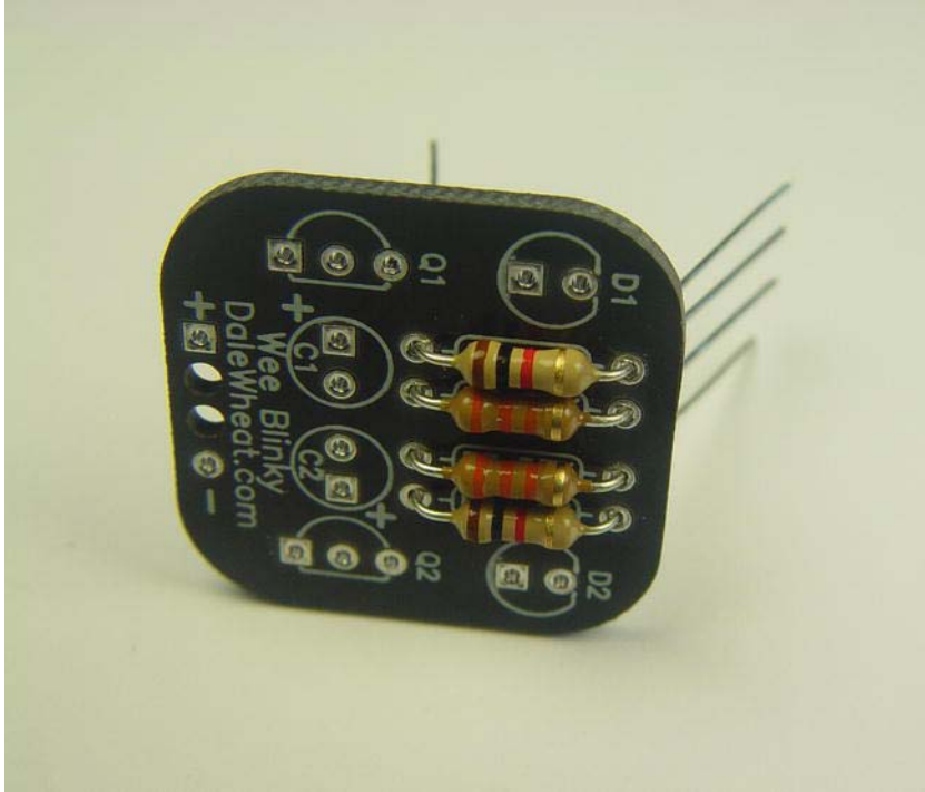
Figure 3-10. Resistor leads are bent at right angles and inserted into holes in the PCB to be soldered.
