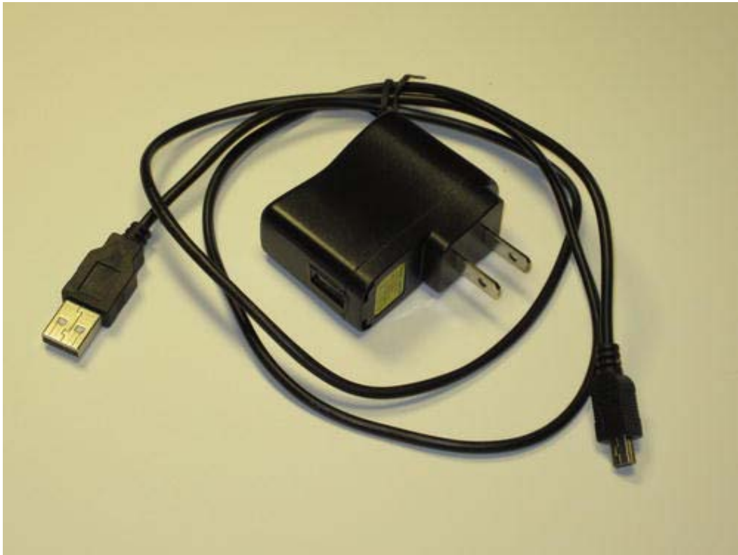
Figure A-2. A USB charger that plugs into the wall and provides a regulated +5V supply. This plug is intended for US wiring, but will operate from 110AC to 240VAC at 50 or 60Hz, which pretty much covers the whole world, if you have the right adapter plug.
