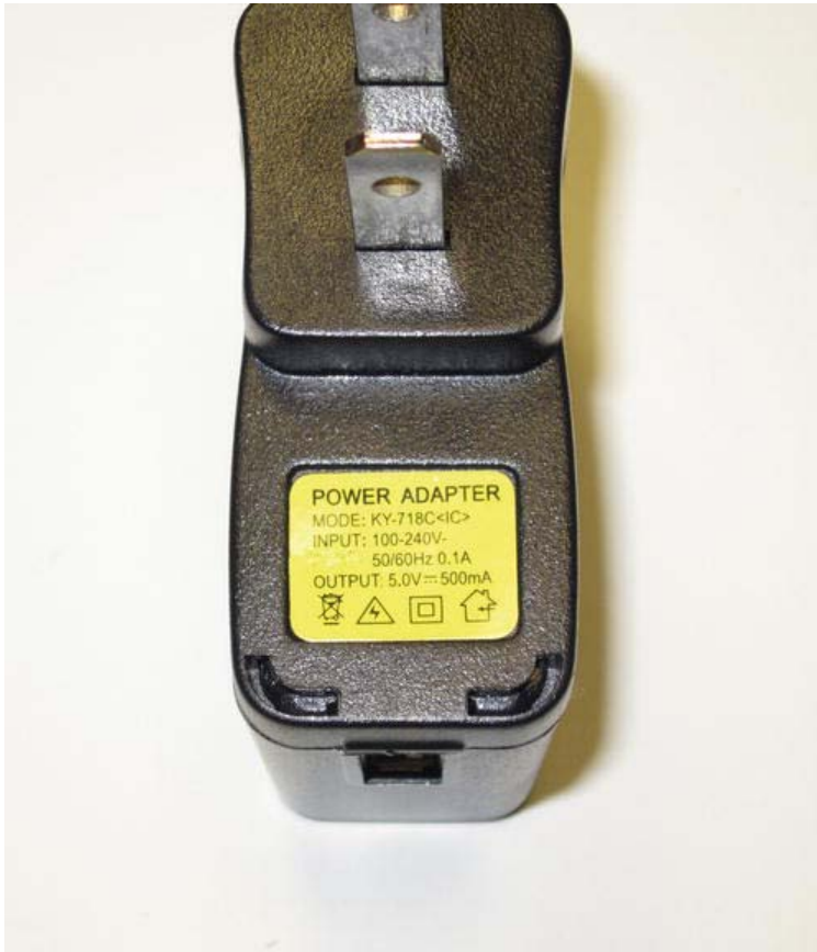
Figure A-3. The label of the USB charger tells us that it accepts anything from 110VAC to 240VAC at either 50Hz or 60Hz. This wide range of input power allows the same internal electronic design to be used worldwide. Only the prongs that plug into the wall vary from location to location. The label also tells us that the USB charger will output +5V at up to 500mA. That's 2.5W!
