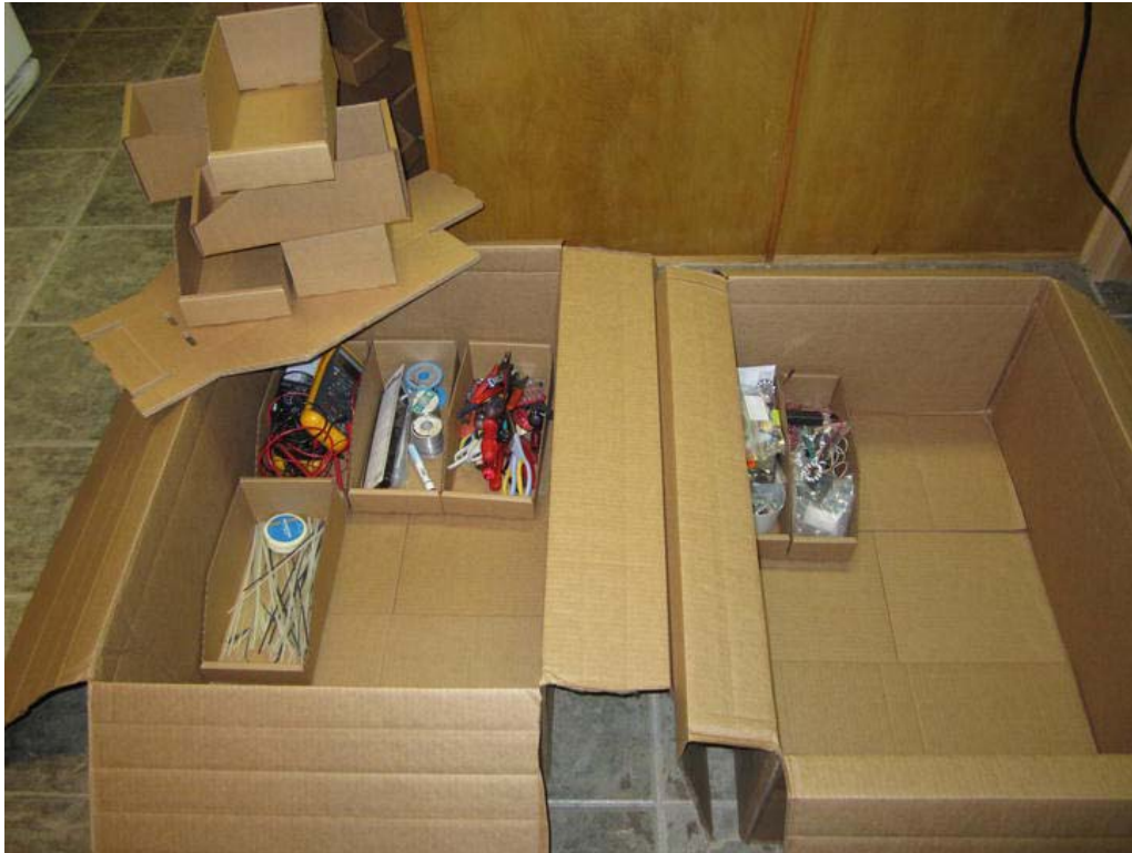
Figure 5-3. Folding cardboard bin boxes help contain some of the smaller bits and pieces during the Big Sort. You can use whatever happens to be available. Some preliminary subsubdivision is going on here. For the most part, the tools are on the left and the components are on the right.
