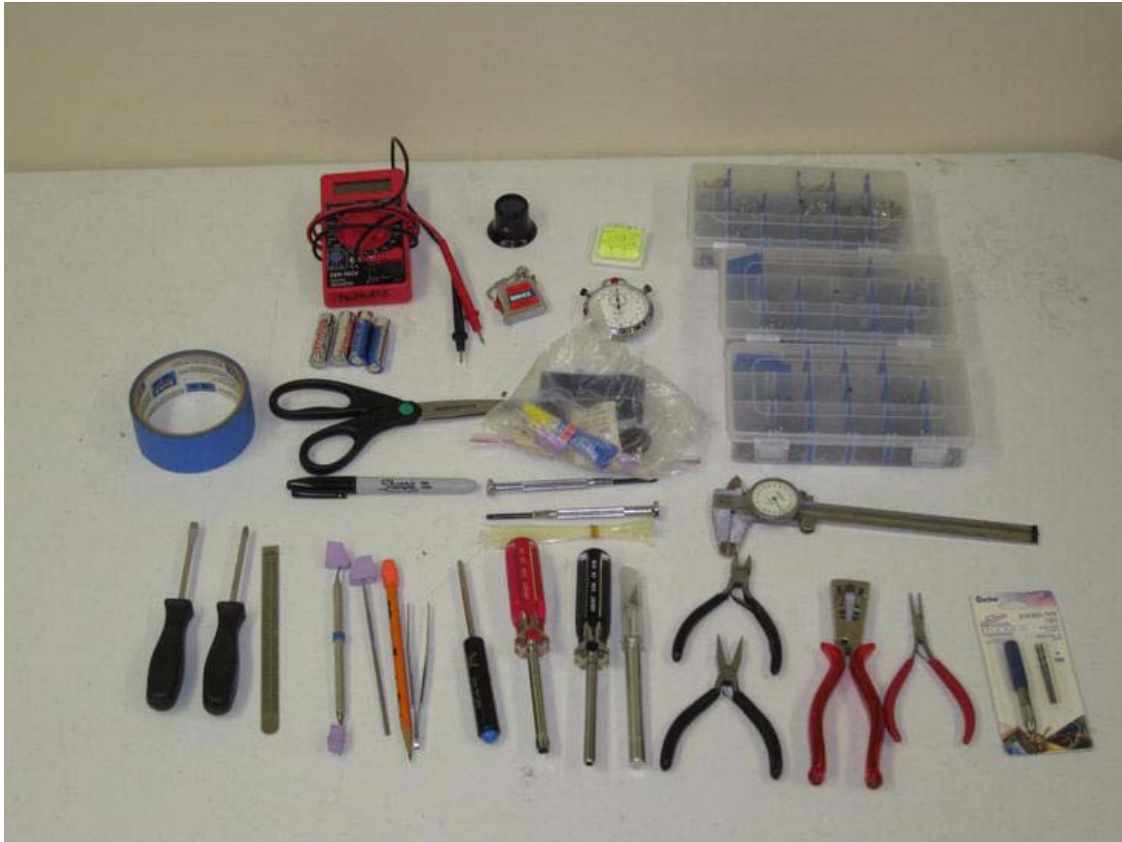
Figure 4-12. The contents of Doug's portable workshop. A variety of hand tools, precision measurement devices, and fasteners (including tape, tie wraps, and super glue) are easily stored in a small tool bag for easy transport. The compartmentalized storage containers at the upper right contain a large assortment of screws, washers, and nuts.
