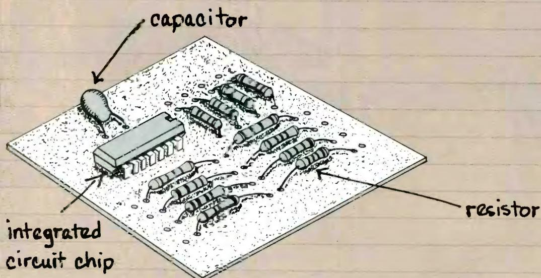
1978-style hardware usually is built of individual parts soldered to a **printed circuit board**. Above, a PC board holds resistors, a capacitor and an IC.
