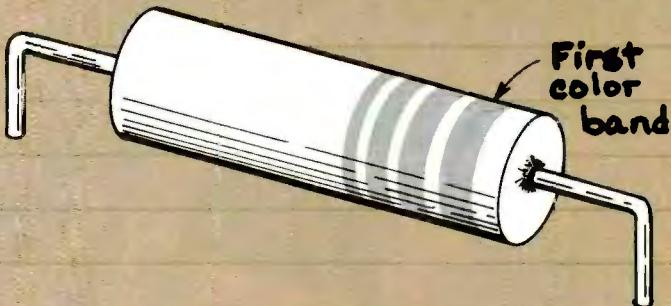
Here are the numbers matching the first two color bands on a resistor. The third band shows the number of zeros following. For example, a 4700 ohm resistor is yellow, violet and red in that order.
