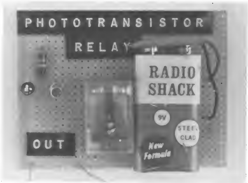
Figure 7-3. The completed light-activated phototransistor relay.
