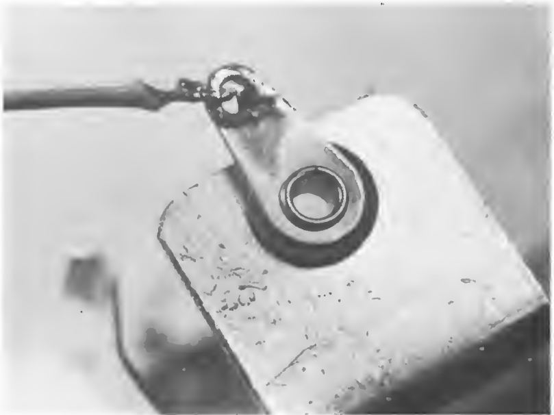
Figure 1-6. A poor solder connection.
