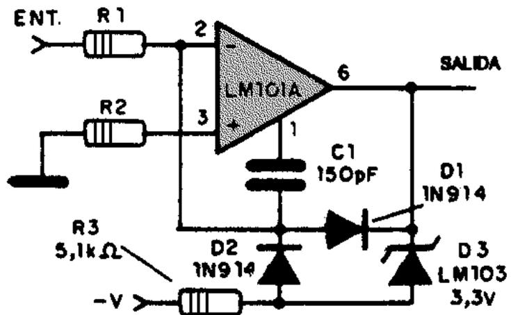
**AMPLIFICADOR PARA TRANSDUCTOR PIEZOELECTRICO**
