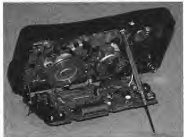
Figure 2-1 A look inside the microcassette recorder.
