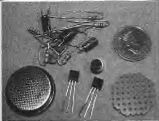
Figure 9-14 Getting ready to miniaturize the ultra sensitive room bug.
