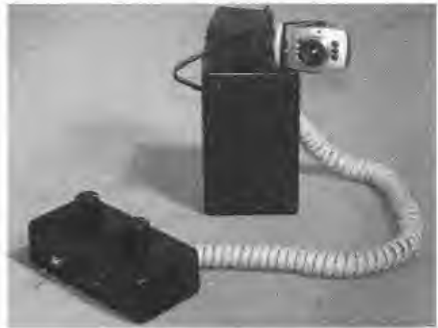
Figure 7-7 The completed manual control box connected to the camera base.
