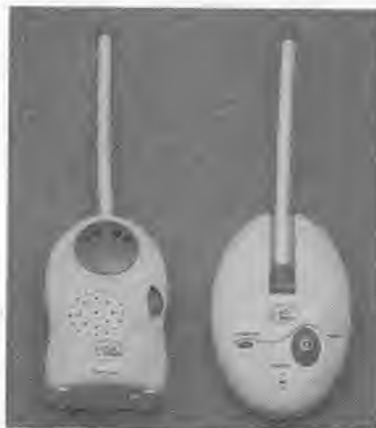
Figure 9.1 A typical baby monitor set. The receiver is on the left and transmitter is on the right.
