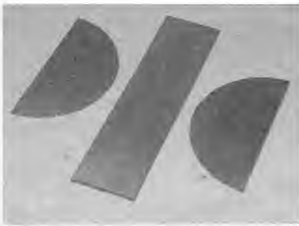
Figure 15-7 The three steel panels that will make up the camera head.
