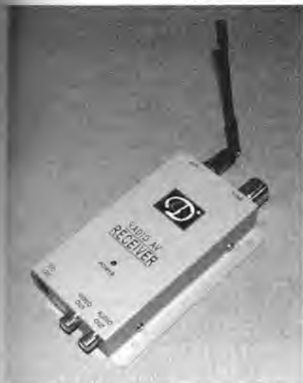
Figure 10-5 A typical wireless video receiver supplied with many transmitter sets.
