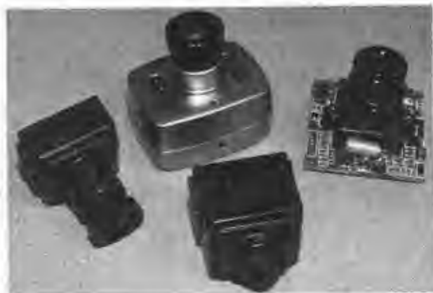
Figure 8-1 A collection of small spy cameras, each with different lux ratings.
