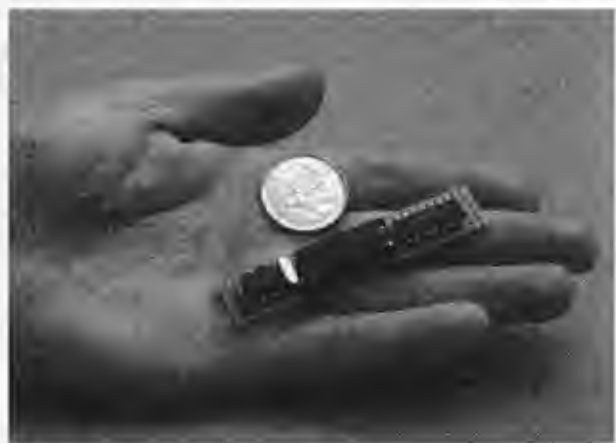
Figure 11-9 The final hardware key logger built on a bit of perf board.
