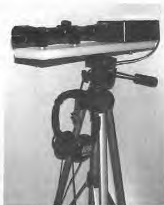
Figure 14-16 The receiver unit is mounted to a tripod for easy alignment.
