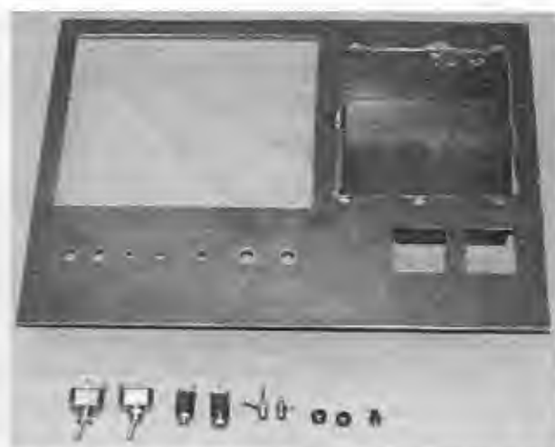
Figure 15-25 A dashboard made of steel sheet for the remote base station.
