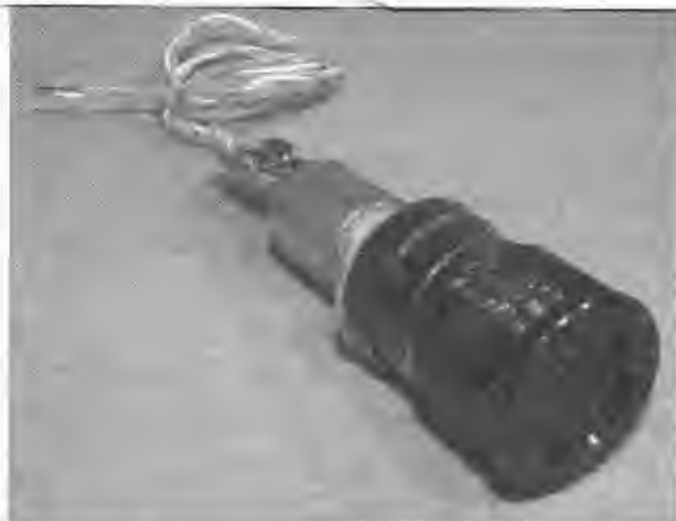
Figure 8-18 The laser module is mounted to a focusing lens assembly.
