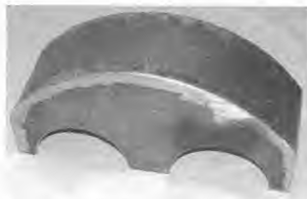
Figure 15-6 Fully welded, the cover will be ready for the elements.
