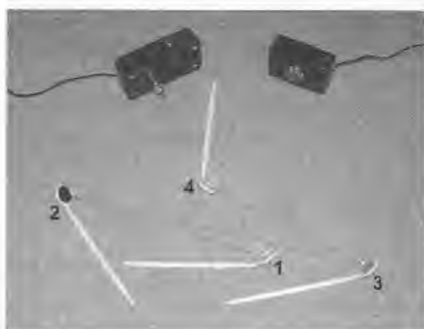
Figure 14-22 A tangled web of laser light is directed by mirrors to the alarm.
