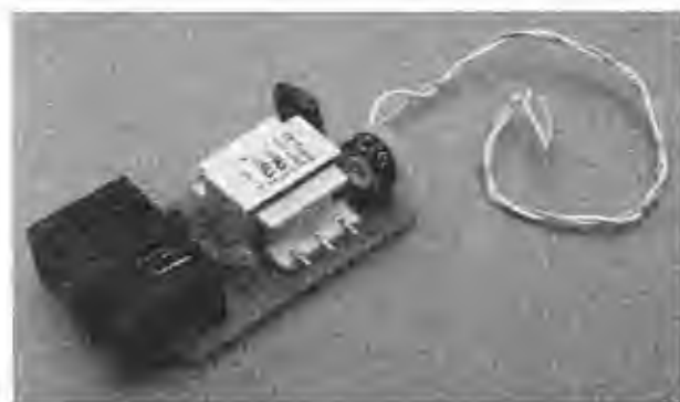
Figure 3-3 The telephone audio interface built on a small perf. board.
