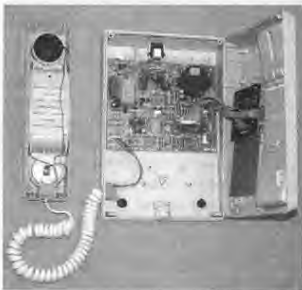
Figure 3-10 Tracing the handset wire back to the telephone’s base.
