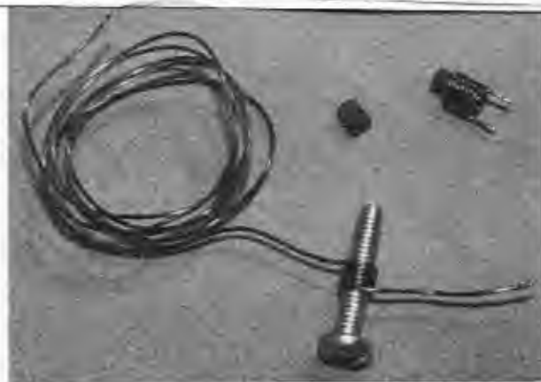
Figure 9-10 Winding a coil around a \frac{1}{8} -bolt. Completed coil also shown.
