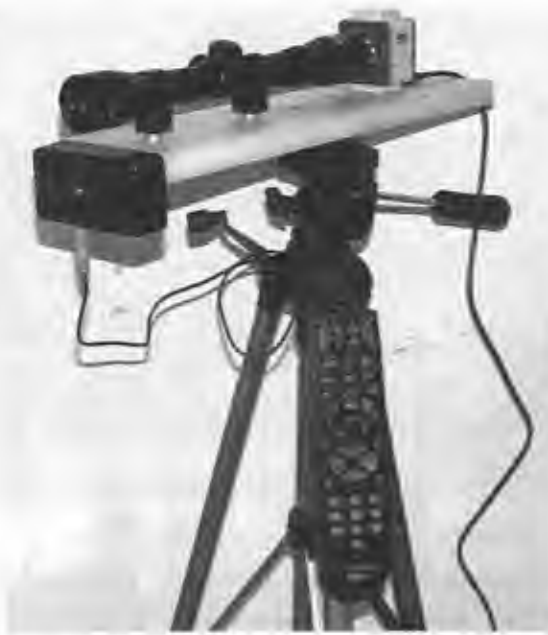
Figure 14-28 A video camera and gun sight make targeting very easy.
