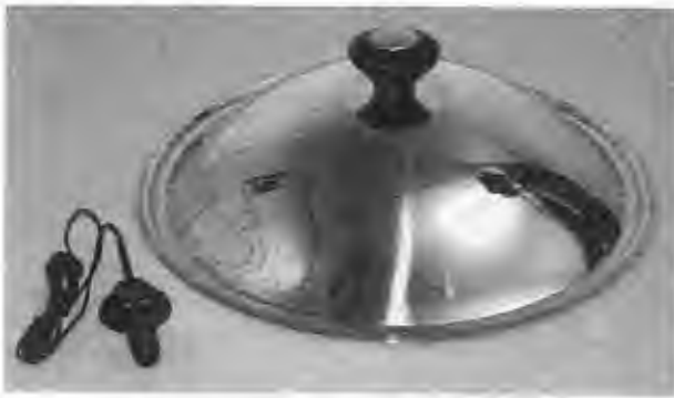
Figure 2-10 A stainless steel wok lid will be used to focus distant sound.
