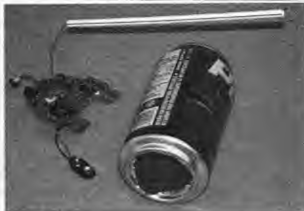
Figure 9-3 A pop can and drinking straw hide the transmitter perfectly.
