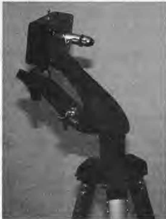
Figure 13-13 The spy camera killer is mounted on a tripod for greater accuracy.
