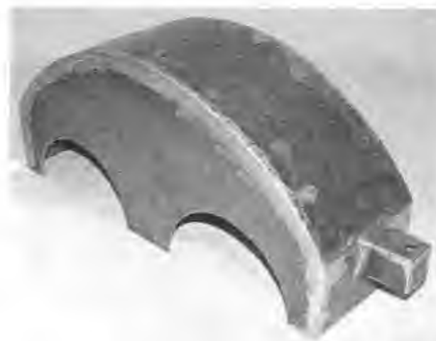
Figure 15-10 The mounting block welded to the ROV cover.
