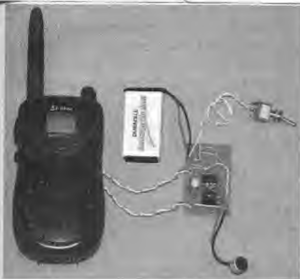
Figure 9-7 Modified radio showing microphone and transmit button extension wires.
