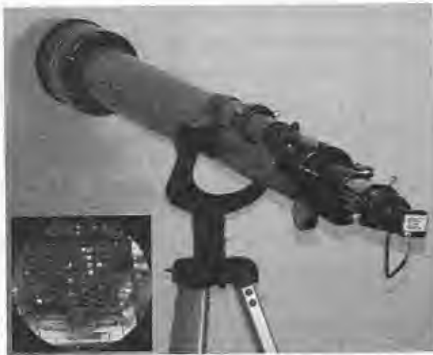
Figure 6-14 Acquiring images at night using a telescope and a very low lux camera.
