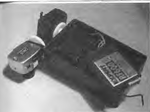
Figure 7-4 The servos and RC receiver are mounted in a plastic box.
