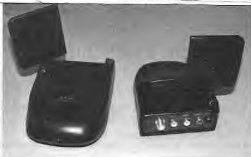
Figure 10-1 A video sender pair for transmitting a video signal around the house.
