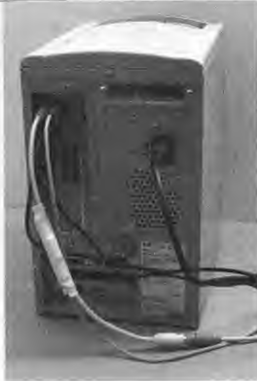
Figure 11-11 Like a chameleon, the HKL blends right in with the other cables.
