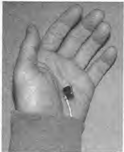
Figure 2-18 The recording trigger switch will be glued into my shirtsleeve.
