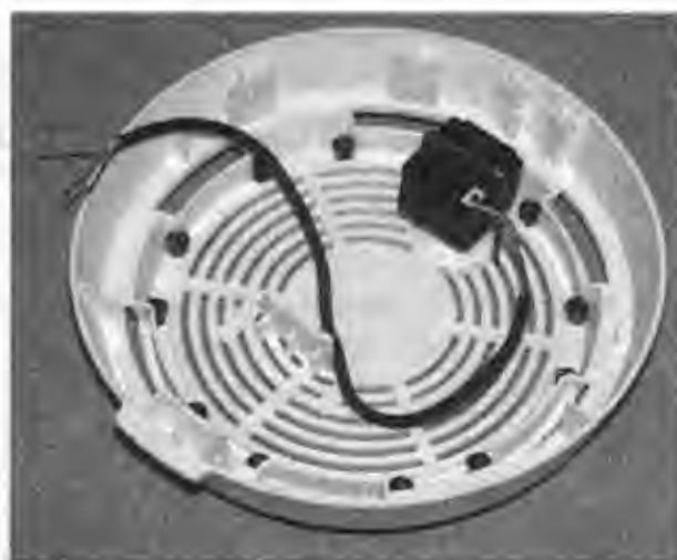
Figure 6-8 Mounting the pinhole camera lens through the test button opening.
