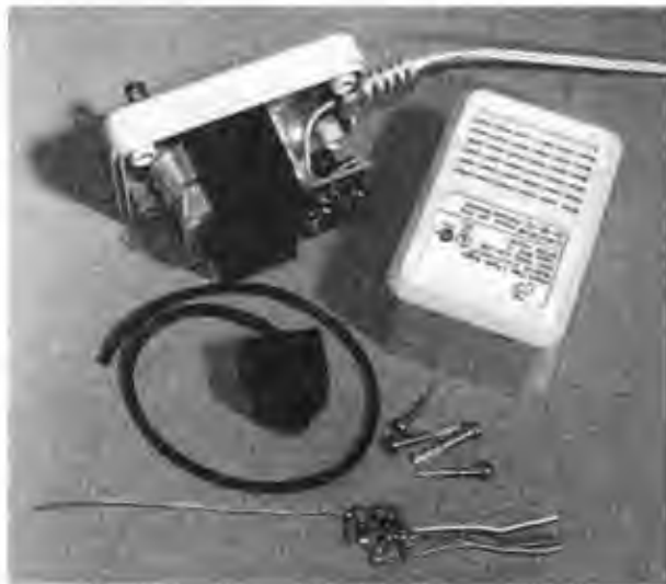
Figure 10-13 Opening the DC adapter to install the camera and transmitter.
