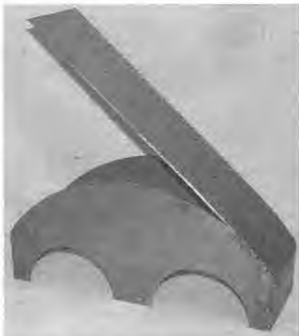
Figure 15-4 Welding the sides and top to form the basic ROV cover.
