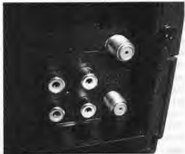
Figure 5-1 The video input/output panel at the rear of a VCR.
