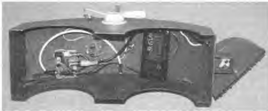
Figure 15-20 Mounting the preamp under the cover with the other electronics.
