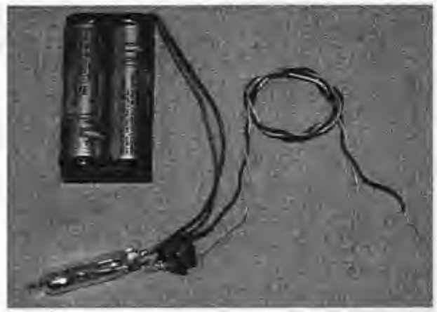
Figure 13-23 A mercury switch will set off the shocker when it is moved.
