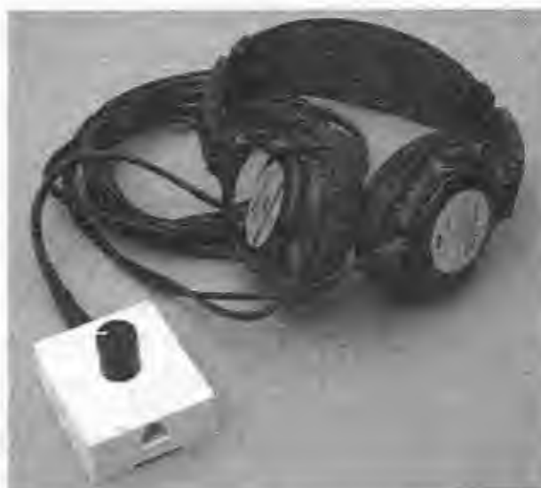
Figure 3-9 The super stealth line tap built into a phone extension box.
