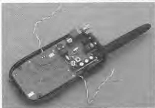
Figure 9-6 Modified radio showing microphone and transmit button extension wires.
