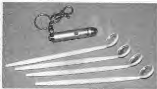
Figure 14-18 A typical laser pointer and some dental mirrors are a few of the required parts.
