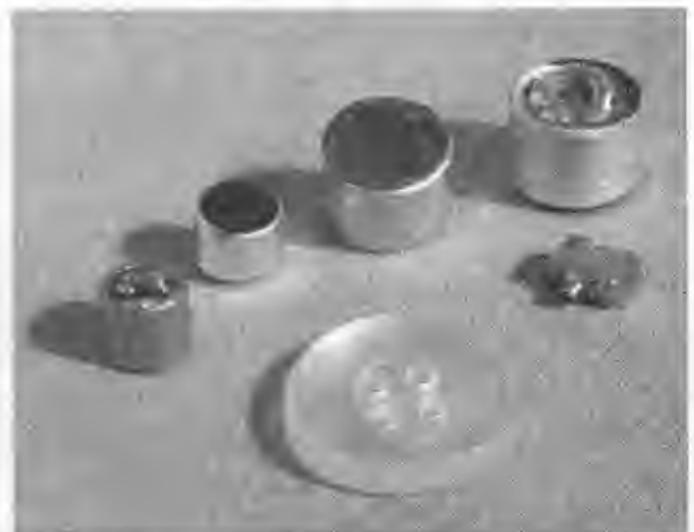
Figure 2-16 A few various sizes of electret microphone elements.
