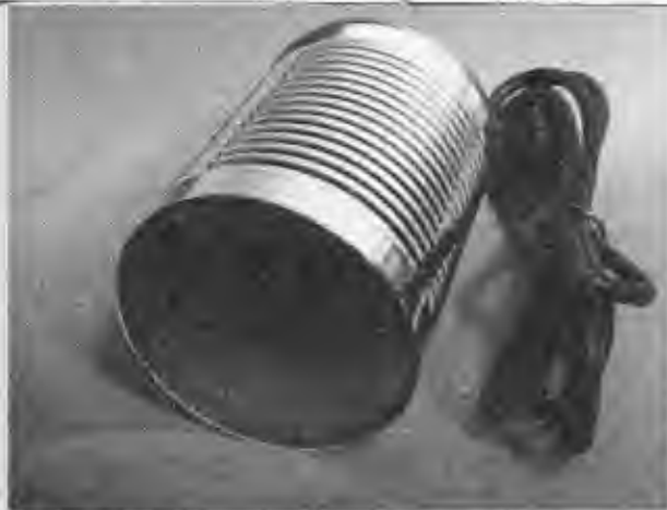
Figure 8-12 My outdoor "soup can" illuminator ready to go to work.
