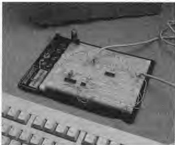
Figure 11-8 Hardware key logger built on a prototyping breadboard.
