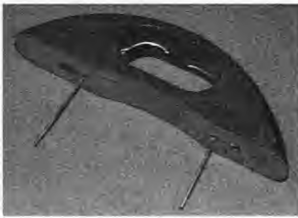
Figure 13-22 High voltage output terminals built into a dresser drawer handle.
