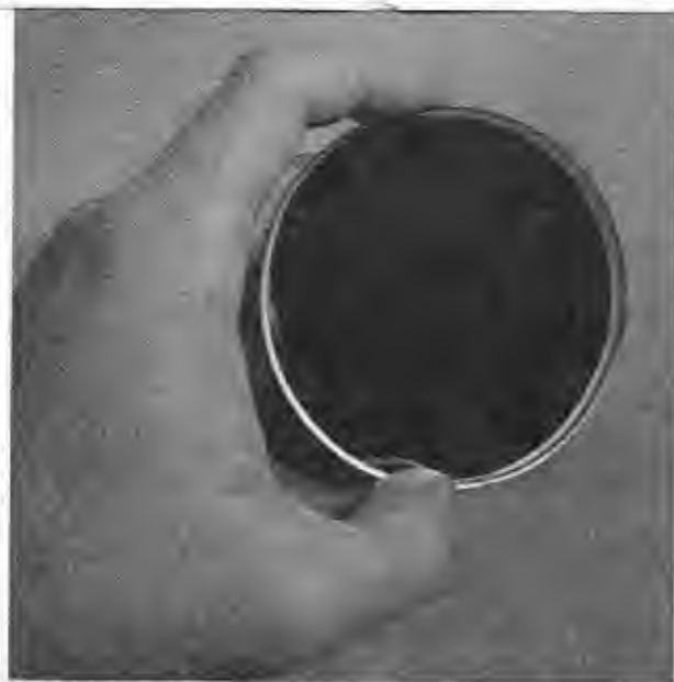
Figure 8-10 A small disc shaped infrared pass filter made from glass.
