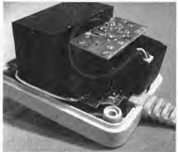
Figure 10-14 Fitting the camera and transmitter into the DC adapter case.
