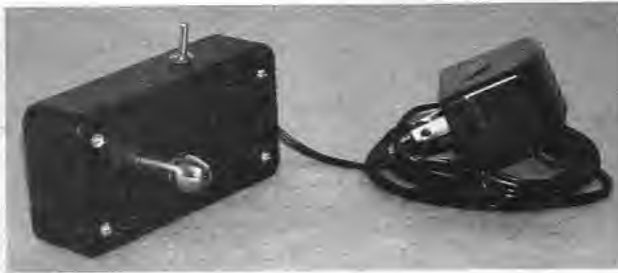
Figure 14-19 The laser pointer will run continuously from an AC adapter.
