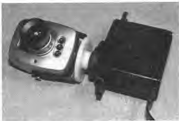
Figure 7-2 Mounting the camera to the first servo along the X-axis.
