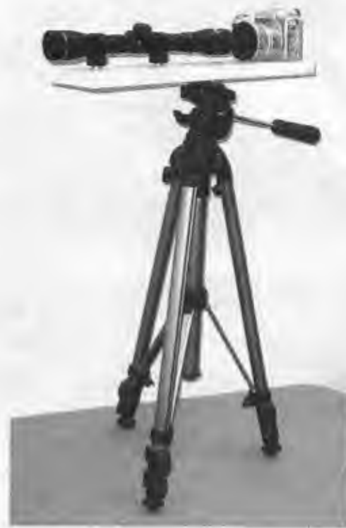
Figure 4-11 Camera and gun sight mounted to a strip of nylon plastic.
