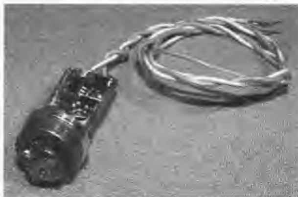
Figure 8-16 A hacked green laser pointer reduced to the diode and driver board.
