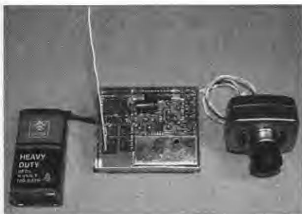
Figure 10-3 The hacked video sender is reduced to its bare essentials.
