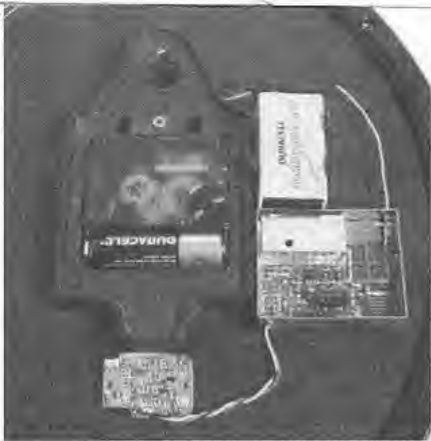
Figure 10-18 The camera, transmitter and battery mounted behind the wall clock.
