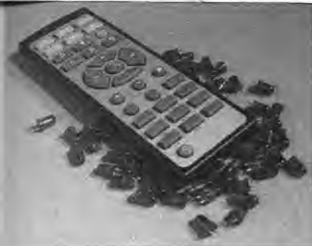
Figure 8-3 A typical infrared remote control and the LEDs that make it function.
