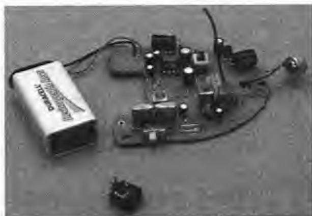
Figure 9-2 Gutting the transmitter to the bare essentials to reduce its size.
