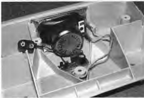
Figure 13-7 White noise generator built right into an old speaker cabinet.
