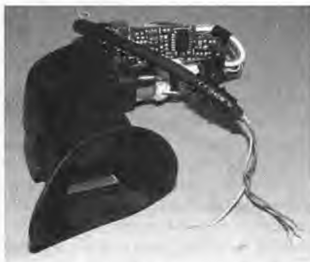
Figure 8-21 A black and white viewfinder hacked from an old camcorder.
