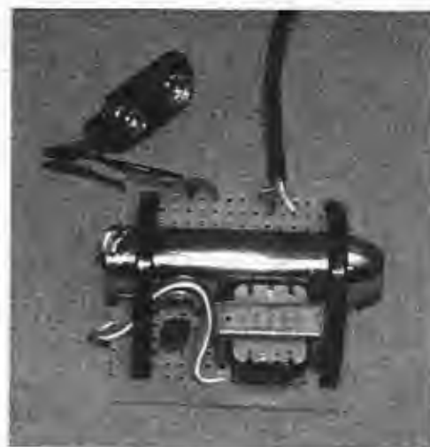
Figure 14-8 The laser beam transmitter built on a small square bit of perf board.
