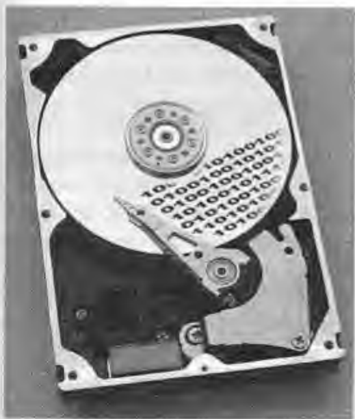
Figure 11-3 A typical 3.5-inch hard disk drive platter.
