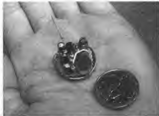
Figure 9-16 A very small bug complete with battery ready for action.
