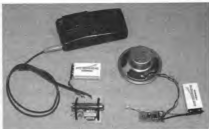
Figure 14-11 Short-range testing. Transmitter shown on the left, and receiver on the right.
