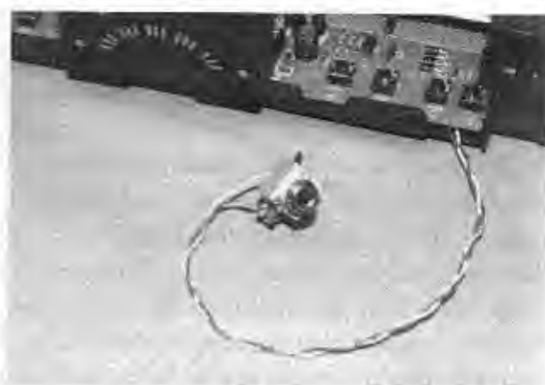
Figure 5-3 Installing a two-conductor jack directly to the pause button.
