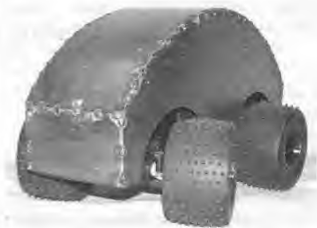
Figure 15-5 Even when only tack welded together, the new cover is very sturdy.
