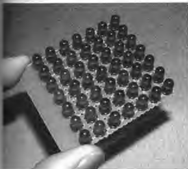
Figure 8-6 A simple 7×7 infrared array that can run from a 9-volt battery.
