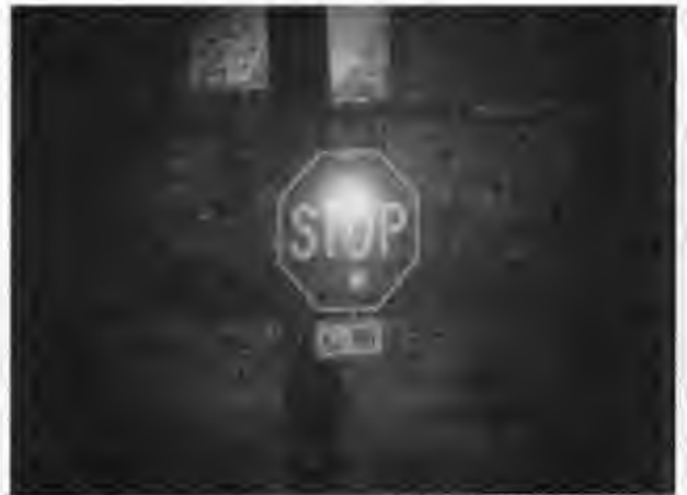
Figure 14-5 The red laser beam lights up a stop sign from well over 1000 feet.
