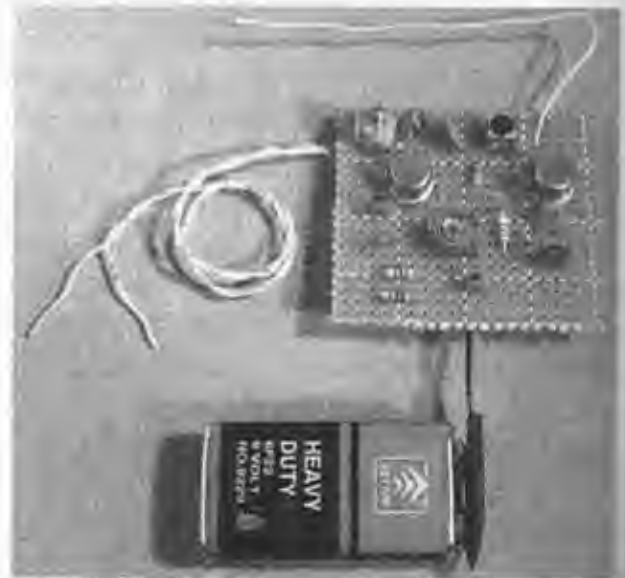
Figure 10-9 The audio video transmitter built on a piece of perf board for testing.
