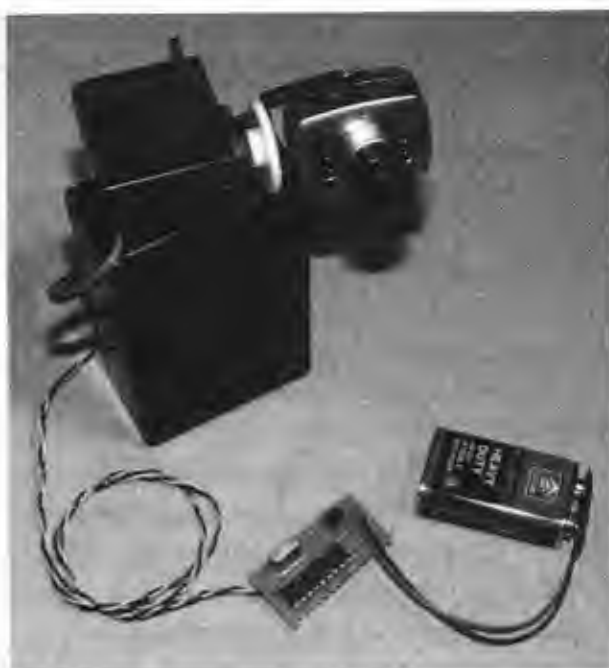
Figure 7-9 The microcontroller activating the pan and tilt camera base.
