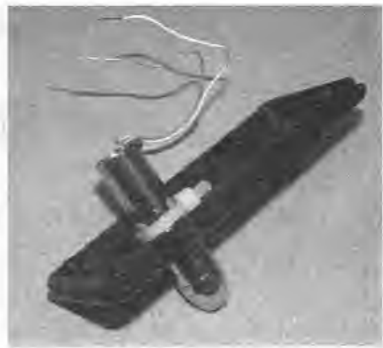
Figure 14-2 The laser pointer with external power leads attached.
