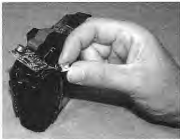
Figure 4-3 Removing the tiny trigger switch from the digital camera.
