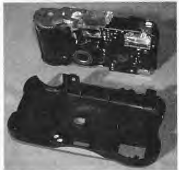
Figure 13-15 Remove the front and rear covers to expose the circuit board.
