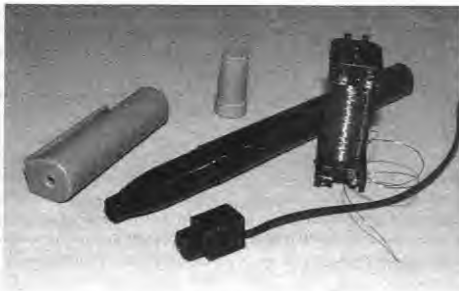
Figure 6-10 A microcamera with pinhole lens will fit into the marker lid.
