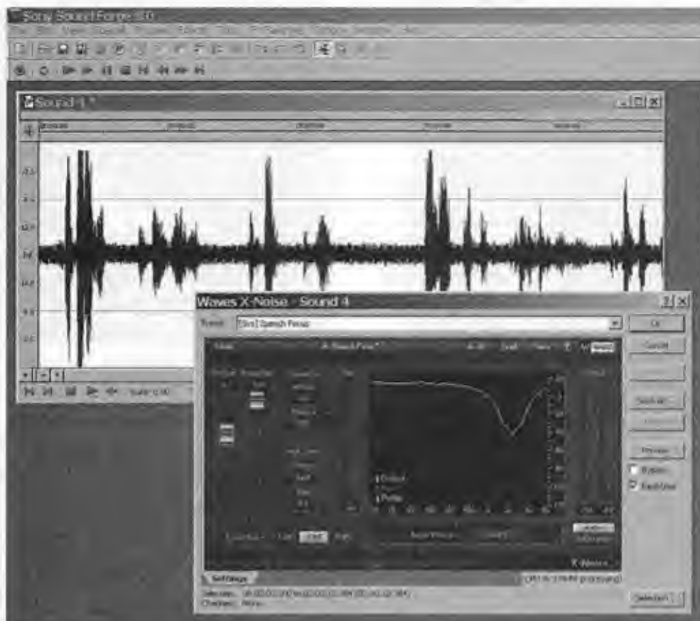
Figure 2-15 A good audio filter can perform magic on your noisy audio source.
