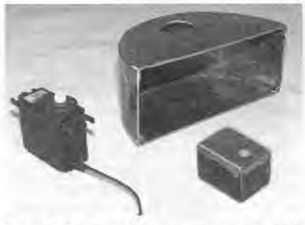
Figure 15-8 The welded camera head, mounting block and servo.
