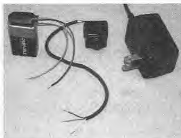
Figure 6-2 A micro camera with pigtail connector shown with two power sources.
