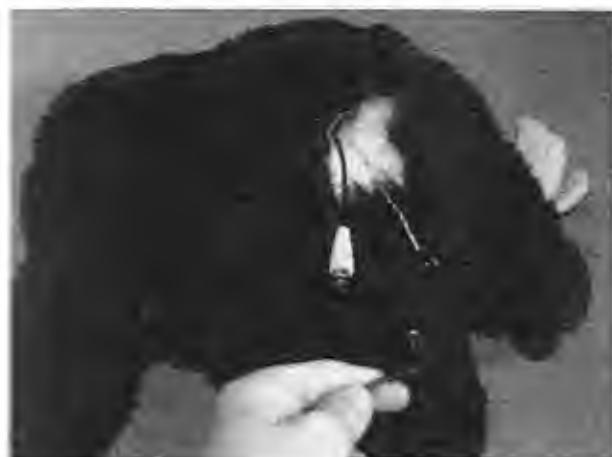
Figure 6-4 Installing video and power connectors into a stuffed toy animal.
