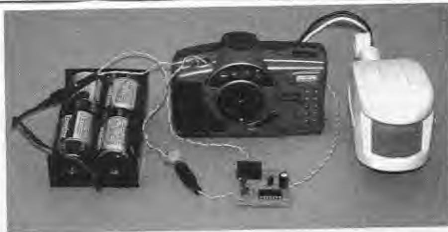
Figure 4-10 Motion sensing camera trigger schematic.
