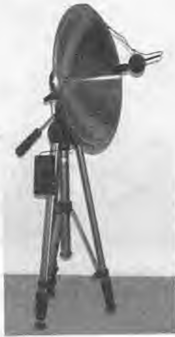
Figure 2-12 The parabolic microphone is mounted on a tripod for stability.
