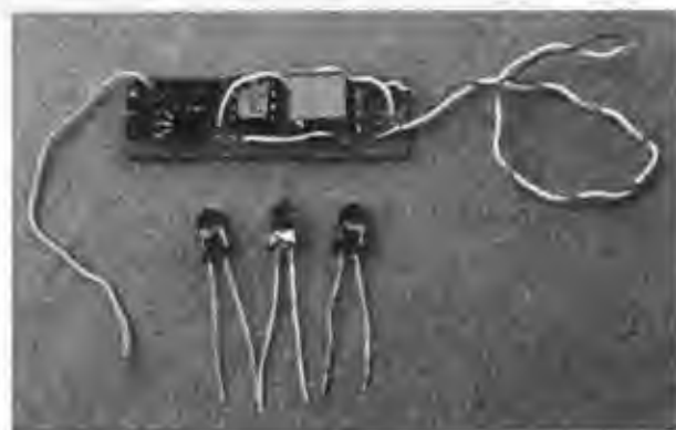
Figure 13-10 Infrared jammer circuit board and LEDs.
