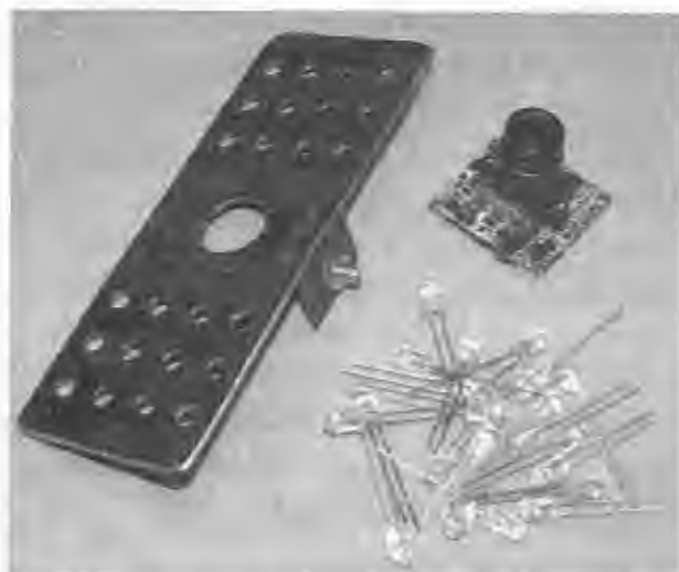
Figure 15-12 The front panel drilled, and ready for camera and LEDs.
