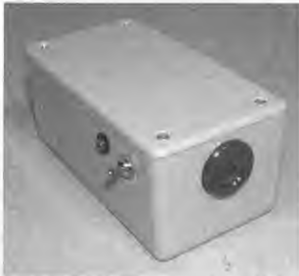
Figure 8-19 The high-power infrared laser illuminator ready for action.
