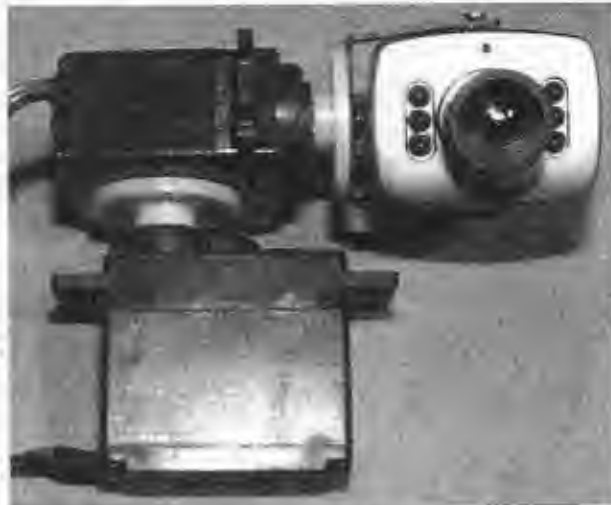
Figure 7-3 Both servos are connected together to form the pan and tilt base.
