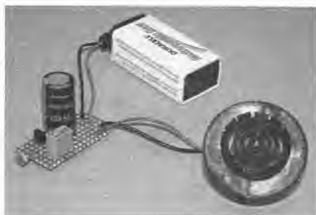
Figure 14-21 The laser perimeter alarm device uses a photocell for detection.
