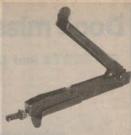
A nibbling tool is used for making cutouts in sheet metal panels.
