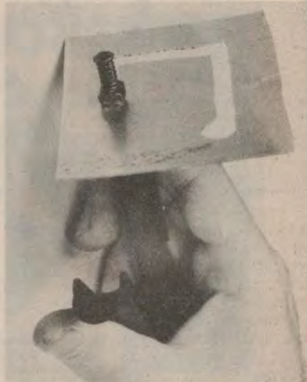
A nibbling tool is used for making cutouts in sheet metal panels.
