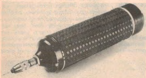
Left: this small battery-powered drill is especially useful for drilling holes in printed circuit (PC) boards. Suitable drill sizes for PC work are 0.8mm and 1mm.
