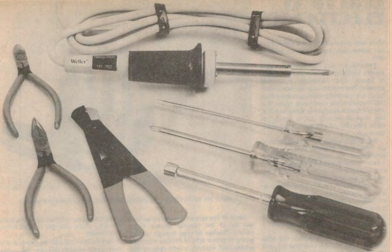
Buy the tools separately if you prefer. Included here are side cutters, long nose pliers, wire strippers, a nut runner, Phillips head and blade screwdrivers, and a 25W soldering iron.
