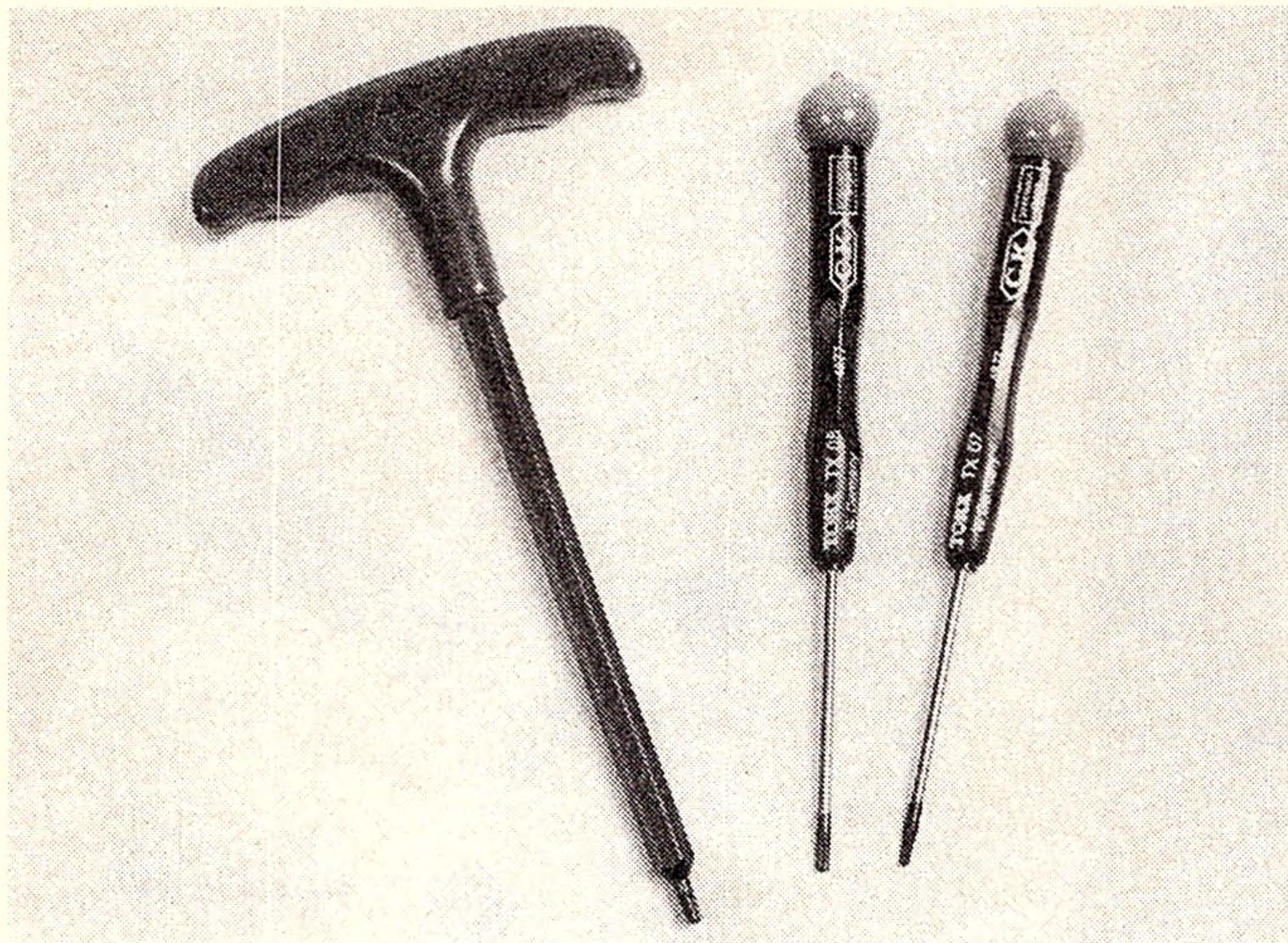
At left is a T-handled Torx screwdriver from Arista which is needed if you wish to gain access to an Apple Macintosh. The other small Torx drivers are from Geoff Wood Electronics.
