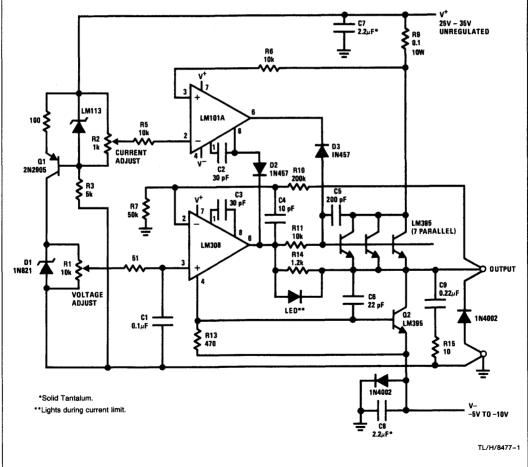
the overall gain set at 5 by the ratio of R10 to R7. An additional LM395 is driven from the negative power supply lead of the LM308 to provide some output current sink capability (2A) so the supply can be quickly programmed even with large capacitive loads. Frequency compensation is achieved with C3 for the LM308 and C4 for the overall loop. Resistor R11, capacitors C5 and C6 and network R15-C9 suppress parasitic high frequency oscillations.
