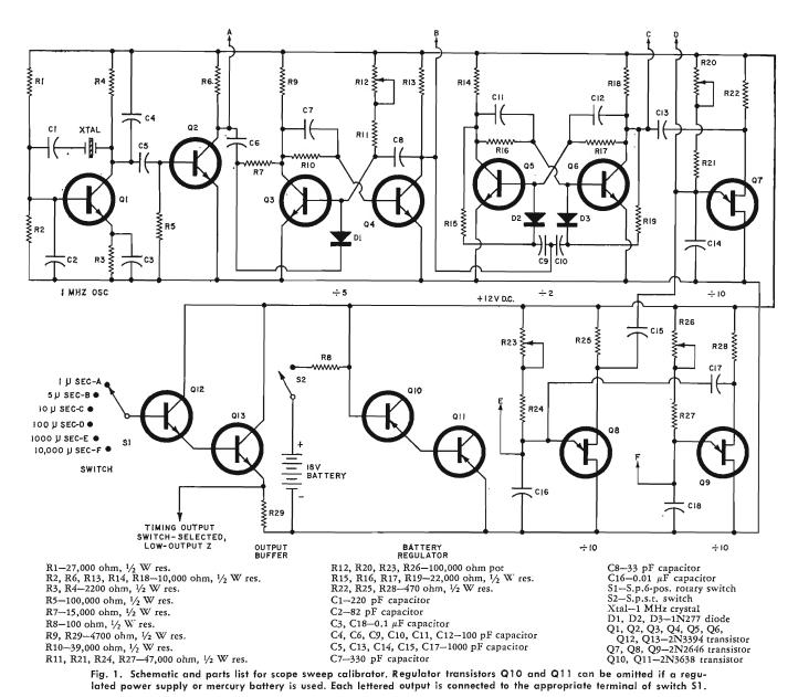
quency of 10 kHz. Both C15 and R25 should be connected since they present a load to Q7. Potentiometer R20 is adjusted until 10 pulses at the Q6 collector result in one sawtooth at the emitter of Q7, as shown in Fig. 2F. This saw-
