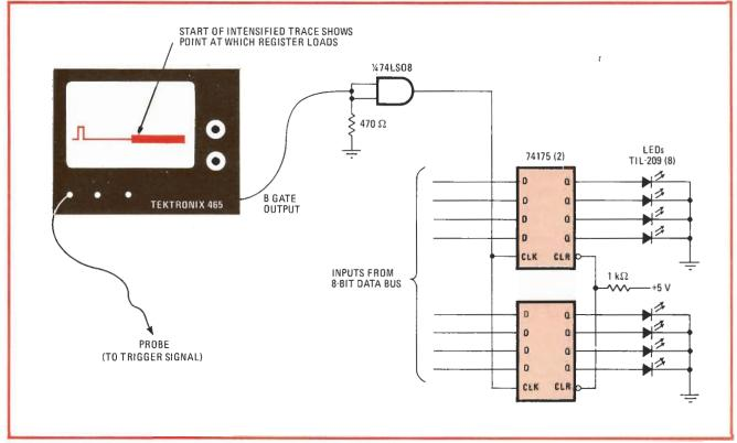
**Rudimentary logic analyzer.** A lit light-emitting diode shows a logic 1 on the microprocessor data bus and a dark LED shows a logic 0—both at the moment that is determined by the setting of the delay-time knob on the oscilloscope. Scope trace indicates duration of program loop; the trace becomes brighter at the point where the data sample is loaded into the register to light the LEDs.
