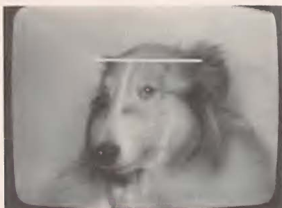
Fig. 4. Here is a typical setup when using the Video Trigger to view a line of video on an oscilloscope. All of the settings for the Video trigger are controlled by a single knob.
