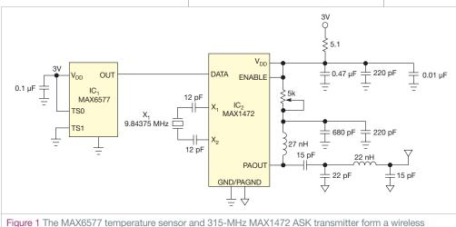
the ambient temperature at the device (**Figure 1**). The output of  $IC_1$  is a square wave with a frequency proportional to temperature in kelvins. ASK transmitter  $IC_2$  modulates the signal onto the carrier frequency of 315 MHz. You
