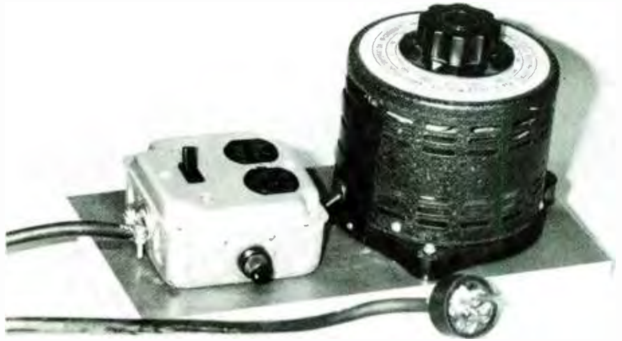
Here's the autotransformer mounted on the board with the electrical box mounted and wired. Note that the fuse holder is easy to reach for fuse replacement.
