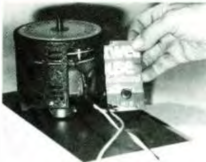
A piece of a two-pound coffee can was used to close up the hole left in the autotransformer's safety shield. The can had an almost perfect curve and indented ribs for reinforcement. A hole was drilled through it. Once the shield was complete, it was sprayed with a flat black paint. After drying, a grommet was installed.
