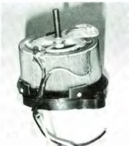
The leads of the cylindrical winding were too short. Colored leads (a red, a black, and a white) were added to make wiring easy and goof-proof. The splices were soldered, and black plastic tape was used to insulate the splices.
