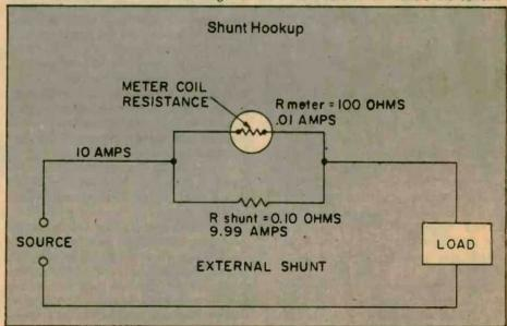
solving Ohm's Law for resistance the proper shunt can be found. This derivation is shown below:
