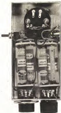
Fig. 7(a) above, shows the method of constructing the simple probe while (b) below, illustrates the location of the few components in the control box and the wiring.
