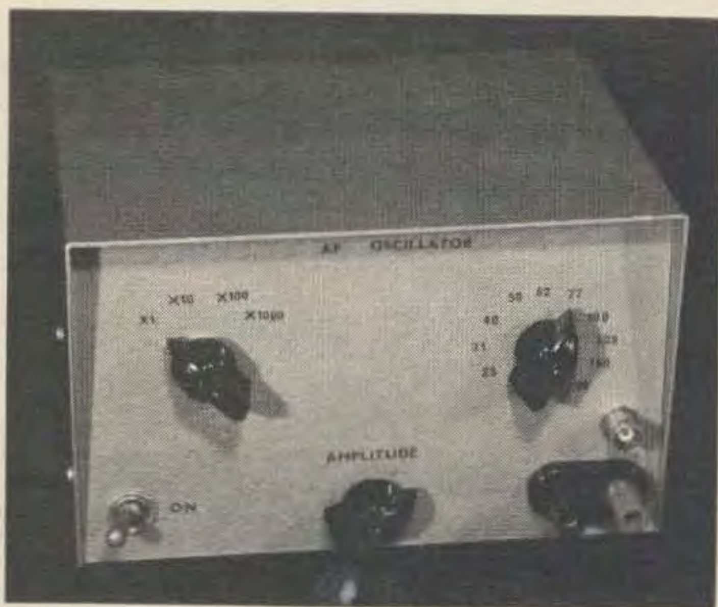
Front view of W6GXN's Wien Bridge audio oscillator.
