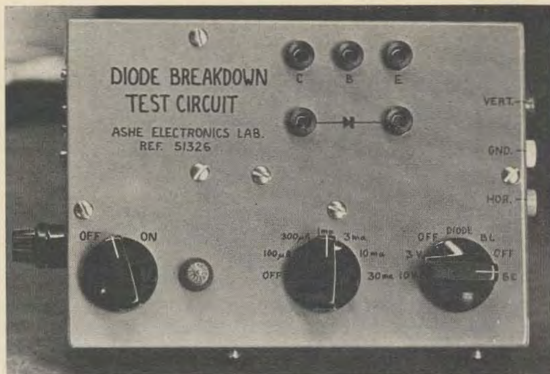
Fig. 5. Top view. I finished the Tester with slow-drying enamel and freehand India ink lettering.
