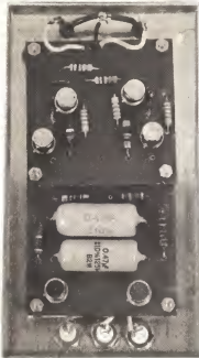
View of the first model of the Transistor Checker in which two boards were bolted together. The test sockets are at the bottom and the LED's at the top.
