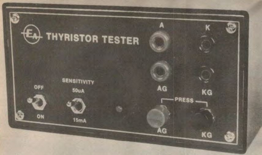
Here is the finished tester, housed in a small plastic utility box. To keep cost down, a LED is used as the test indicator.
