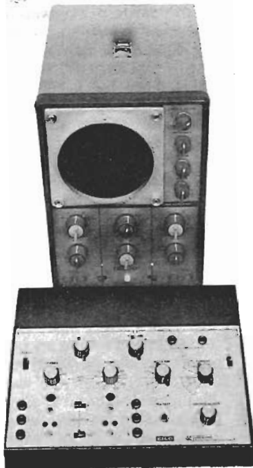
FIG. 1—TRANSISTOR-DIODE CURVE TRACER plugged directly into a scope. The output of this tracer can be displayed on any general-purpose scope.
