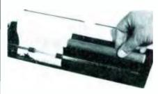
to feed freely. You can count on the paper roll to remain in perfect alignment for a l-o-n-g listing. Like the paper, the dowel fits in the platten groove.
