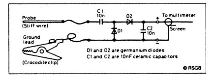
Figure 1 The diode probe can be made from four electronic components
