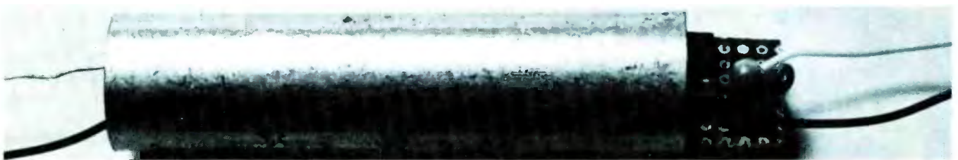
THE PROBE'S PARTS are small enough to mount on a perfbboard that is 7/10-inch wide. The board's length is not critical. There's sufficient space inside most probes to permit mounting of parts. Refer to text for shielding information.
