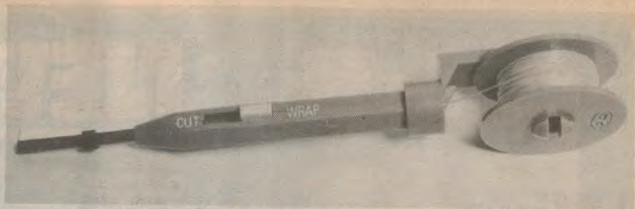
Above & below: the "Just Wrap" from OK Machine & Tool Corporation. The tool wraps insulated wire onto the terminal; terminal corners bite through insulation for electrical contact.
