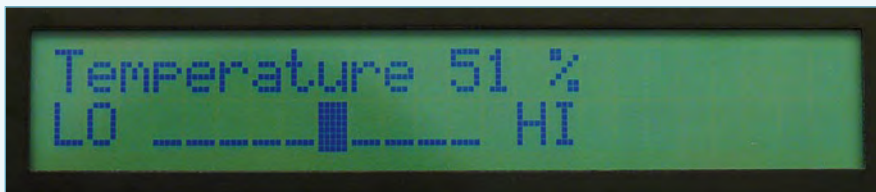
Figure 5. The start menu at power-up shows the soldering iron control.
