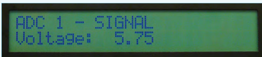
Figure 6. Measurement using channel 1 (range 10 VDC).
