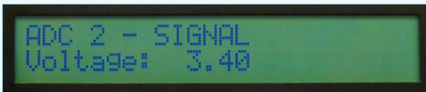
Figure 7. Measurement using channel 2 (range 40 VDC).
