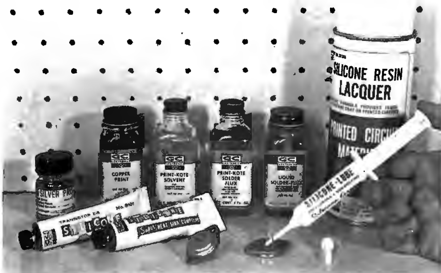
Pc board chemicals include silicone grease heat-sink compounds, conductive paints, silicone resin lacquer board coating and solvent.
