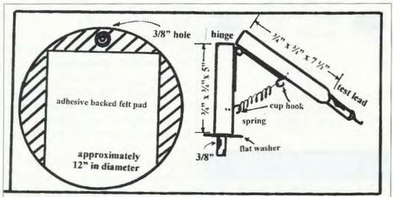
**Fig. 1.** Dimensions of the base and hold-down device are approximate. They were selected to use the wood "stock" I had on hand to match the "hobby hinge," and the base size is the remaining "stiffener" for the pizza pan. The primary requirement is, however, to have the test lead point become usable in the lower half of the working surface.
