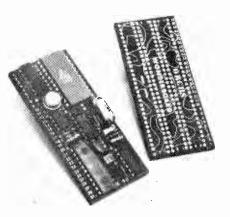
rows of 31 holes. These rows are spaced at 0.3in and the holes are filled with a conductive elastomer.
