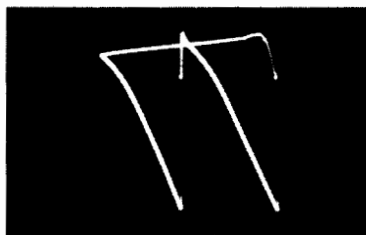
(A) Correct waveform, obtained with low-C probe.
