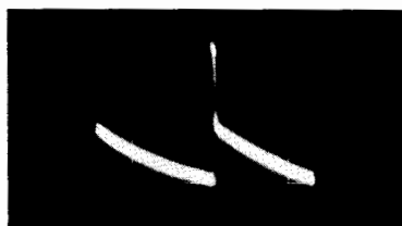
Fig. 7-5. Normal waveform at point D.
