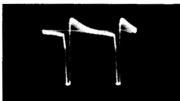
Fig. 5-19. Mixed pulse and sawtooth waveform.
