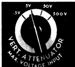
Fig. 1-21. Step attenuator; with maximum input voltages marked.
