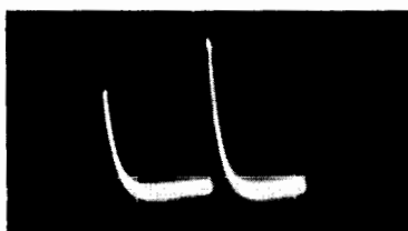
Fig. 7-6. Distorted waveform at point D when capacitor C1 is low in value.
