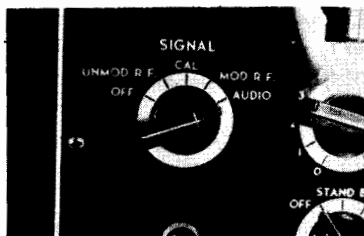
Fig. 8-11. Most signal generators have an audio-frequency output.
