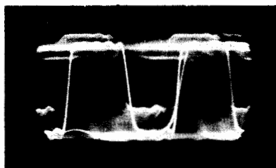
Fig. 1-47. Pattern jumping, caused by fluctuating line voltage.
