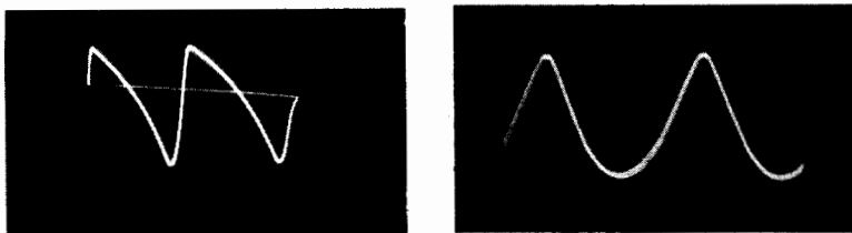
Fig. 9-4. Typical waveforms at filter input.
