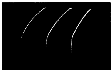
Fig. 7-16. Input waveform to the vertical-blanking network.
