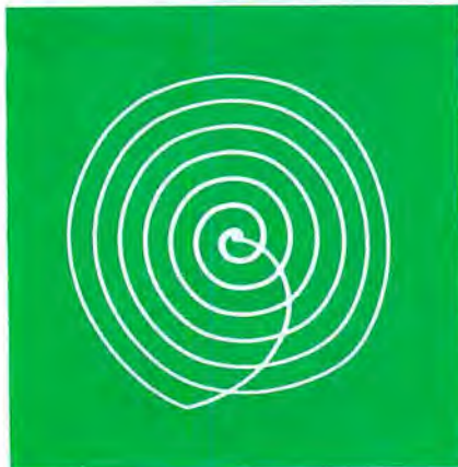
Fig. 9. Pinwheel (A) and spiral (B) patterns are produced by sawtooth waveforms of different frequencies.
