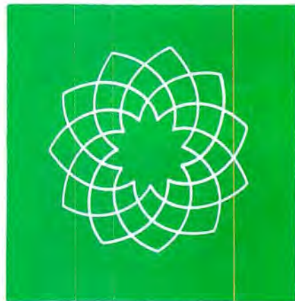
Fig. 12. Frequency comparison with circular sweep. Ratio of triangle to sine sweep is 11:4.
