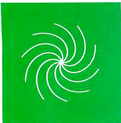
Fig. 9. Pinwheel (A) and spiral (B) patterns are produced by sawtooth waveforms of different frequencies.
