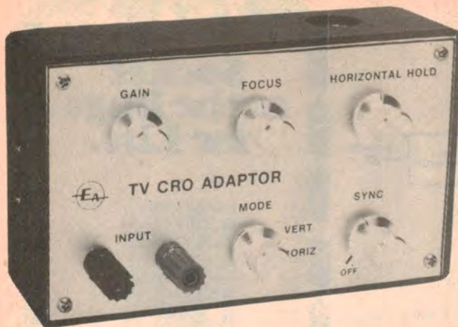
ABOVE & RIGHT: the completed prototype. The unit may be powered either from a 9V battery or from a plugpack power supply.
