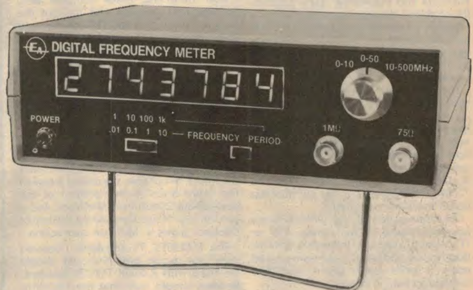
View of the prototype fitted with the optional tilting bail. The 1M \Omega input is used for the 0-10 and 0-50MHz ranges while the 75 \Omega input is used for the 500MHz range.
