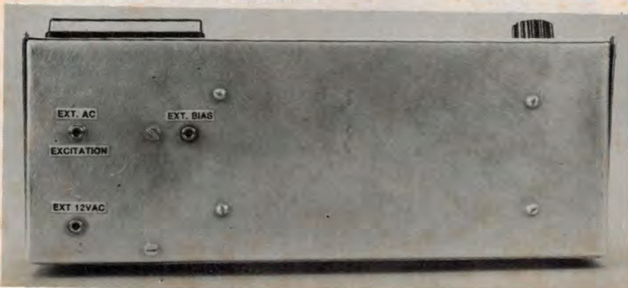
Above: view inside the prototype. Note that a few minor changes were made to the PCB after this photograph was taken. Below is a view of the rear panel. The external bias socket must be isolated from chassis.
